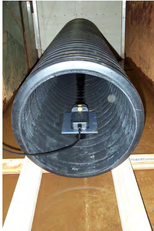
Figure 4. Looking upstream at the SW in plastic pipe section. The SW was positioned 7.5 ft downstream from the pipe entrance.
