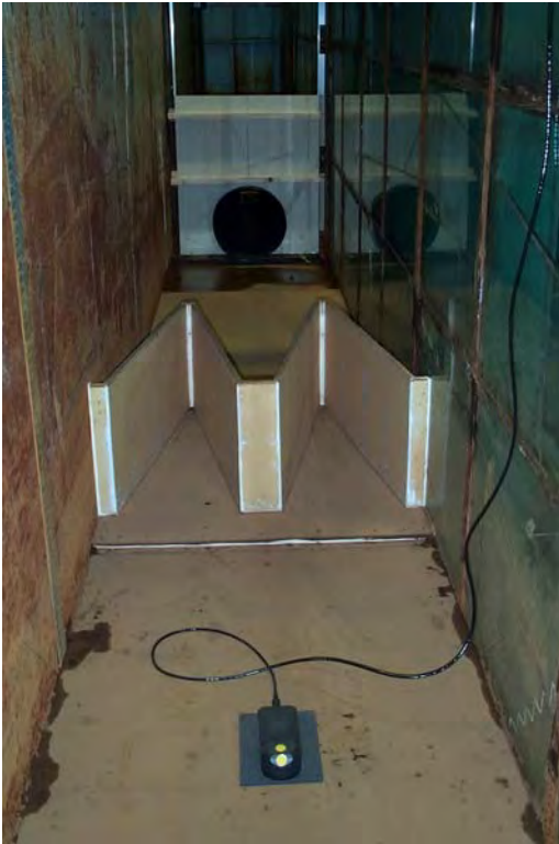
Figure 3. Looking downstream at the SW and the 1.67-ft-high labyrinth weir in the open channel section. The bulkhead entrance to the 18-inch pipe can be seen beyond the labyrinth weir. A staff gage is visible on the steel wall across from the SW transducer.
