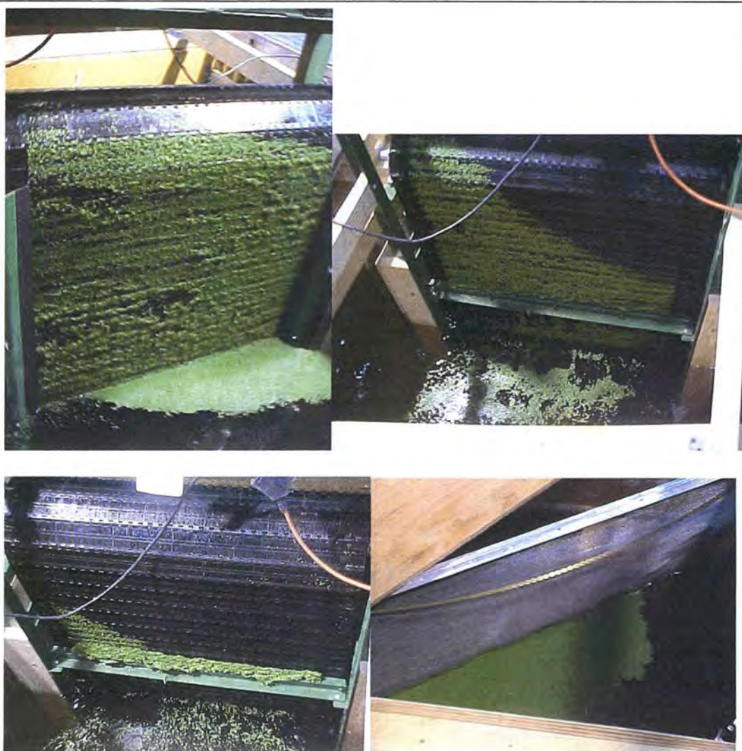
Figure 8. - Duckweed experiments on the original screen. Upper left is the duckweed sticking to the screen (flow from left to right). Upper right is the back side of the screen with the weed washing off with flow through the screen. Lower left is the weed material accumulating on the middle frame support. Lower right is the duckweed that passed by the screen and was captured on the screen upstream from the bypass pipe.
