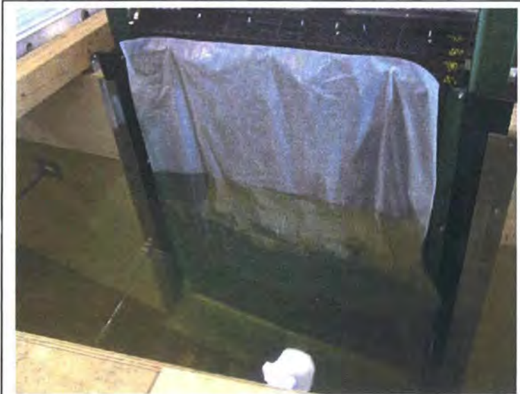
Figure 13. - A double thickness of plastic sheeting was attached to some of the hooks on the face of the screen to hold it in place over the screen and seals for a loading test simulating a debris clogged screen.
