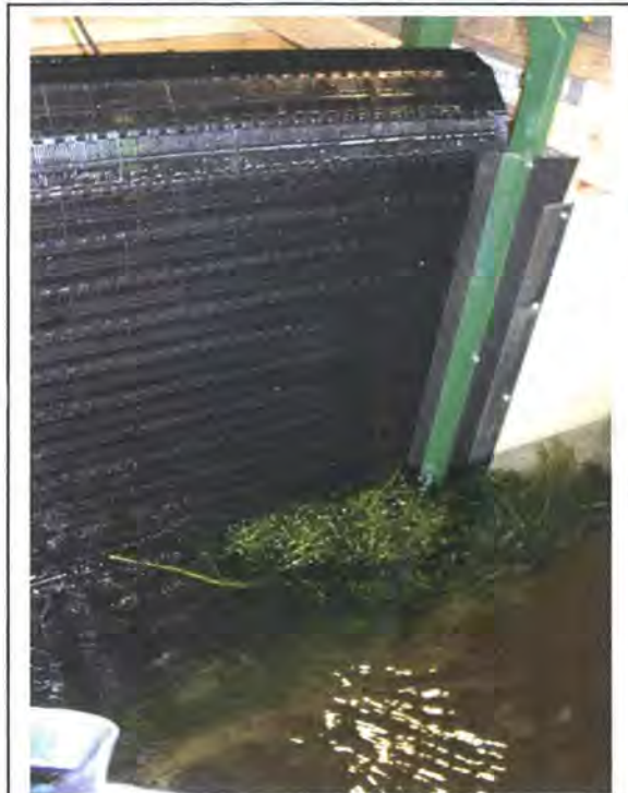
Figure 7. - Egaria weed was released upstream from the screen and “balled up” near the downstream end of the screen before being swept downstream to the bypass. No egaria was captured by the original traveling screen.
