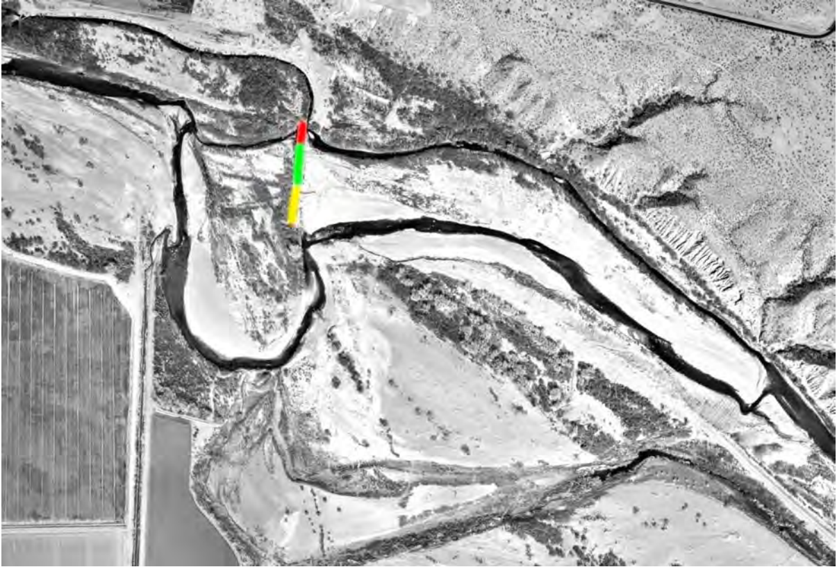
Figure 15. Location of the Graham diversion dam, and potential sections for replacement with rubber inflatable dam or Obermeyer Gate.
