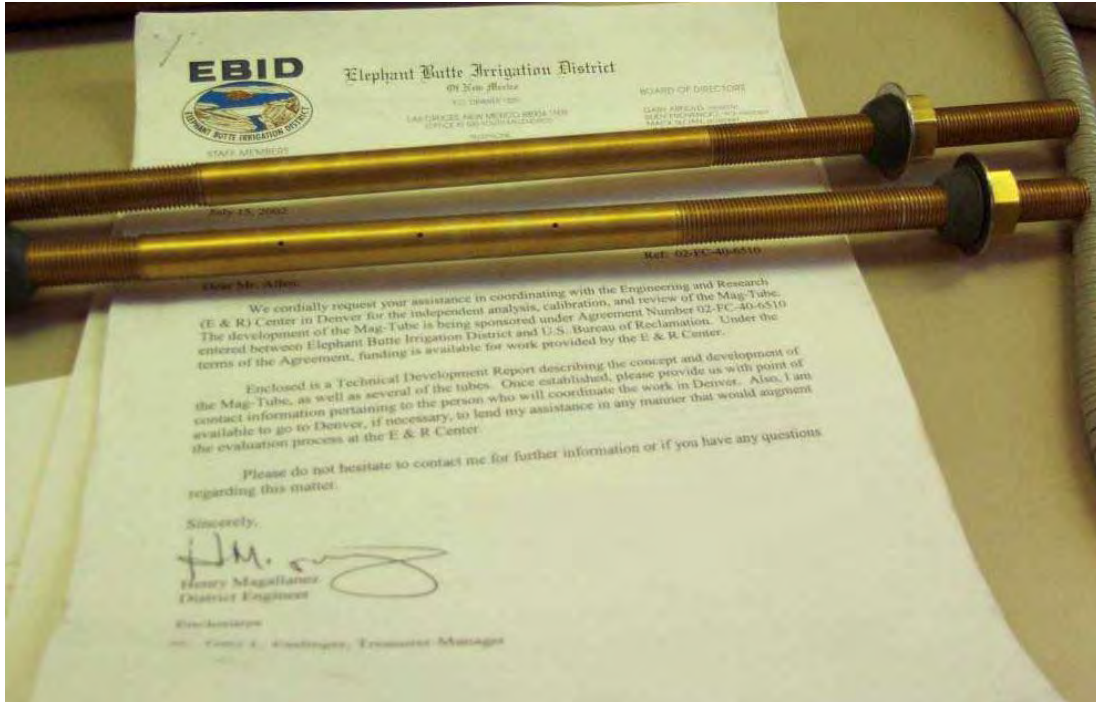
Figure 1. — Prototype Mag-Tube flow meters. Note the three pressure ports on the nearest tube.
