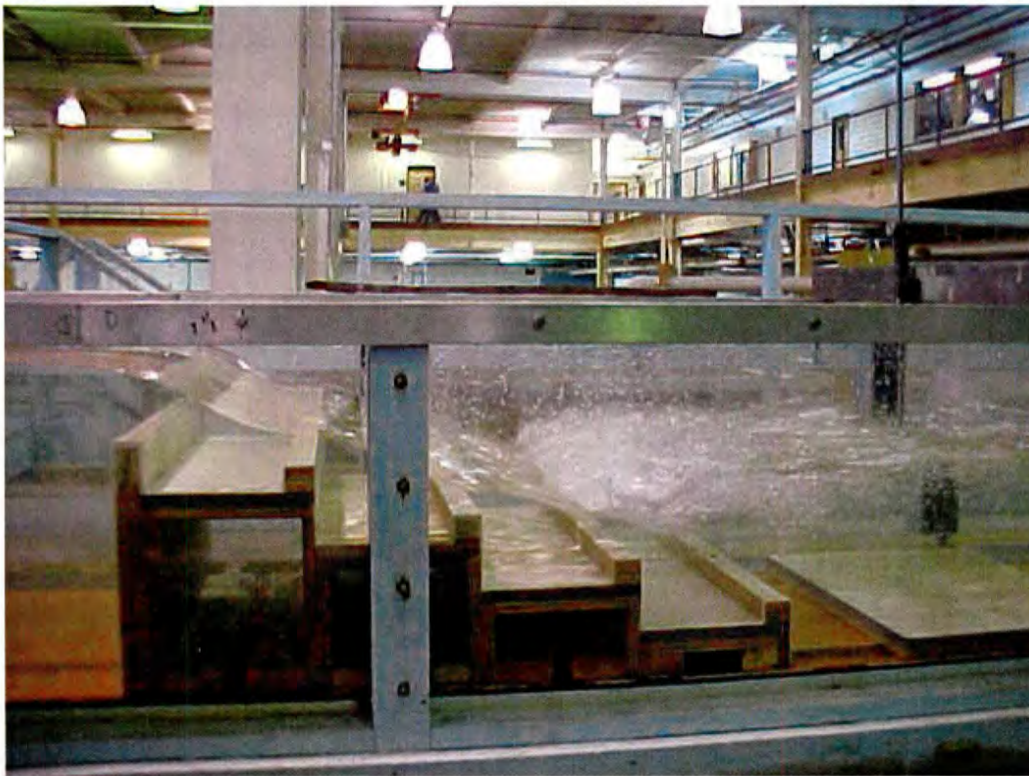
Figure 4: Four foot step length; Q = 330 \text{ ft}^3/\text{s} , TW = 165 \text{ ft}^3/\text{s}
