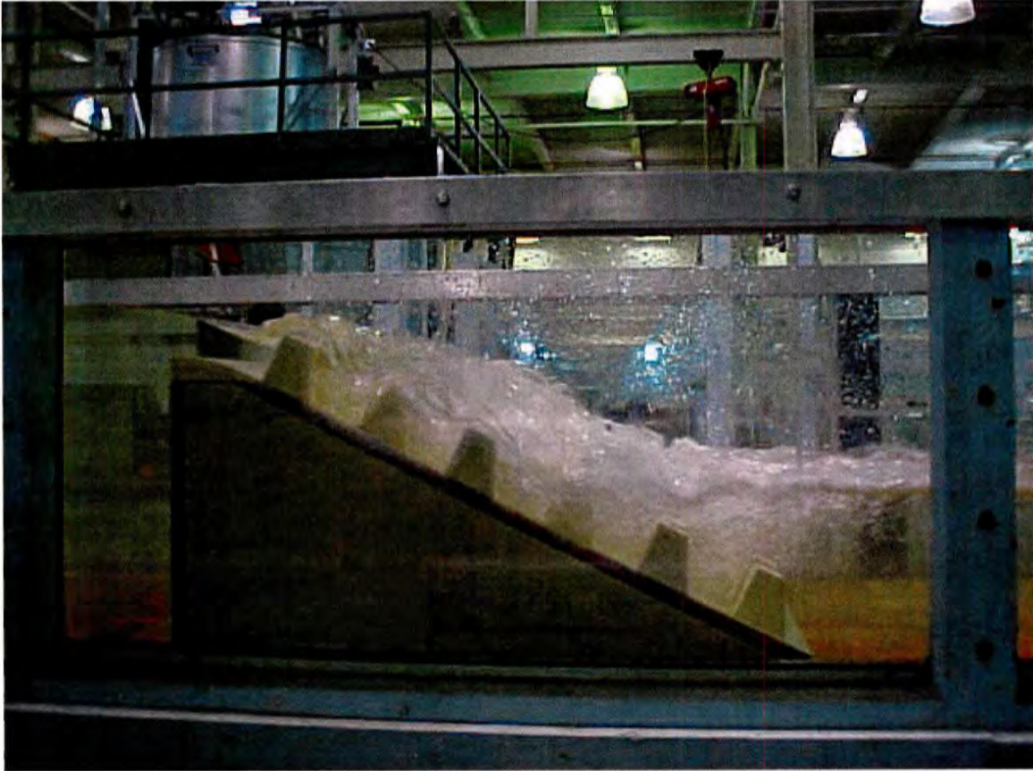
Figure 7: Baffled Apron; Q = 330 \text{ ft}^3/\text{s} , TW = 165 \text{ ft}^3/\text{s}
