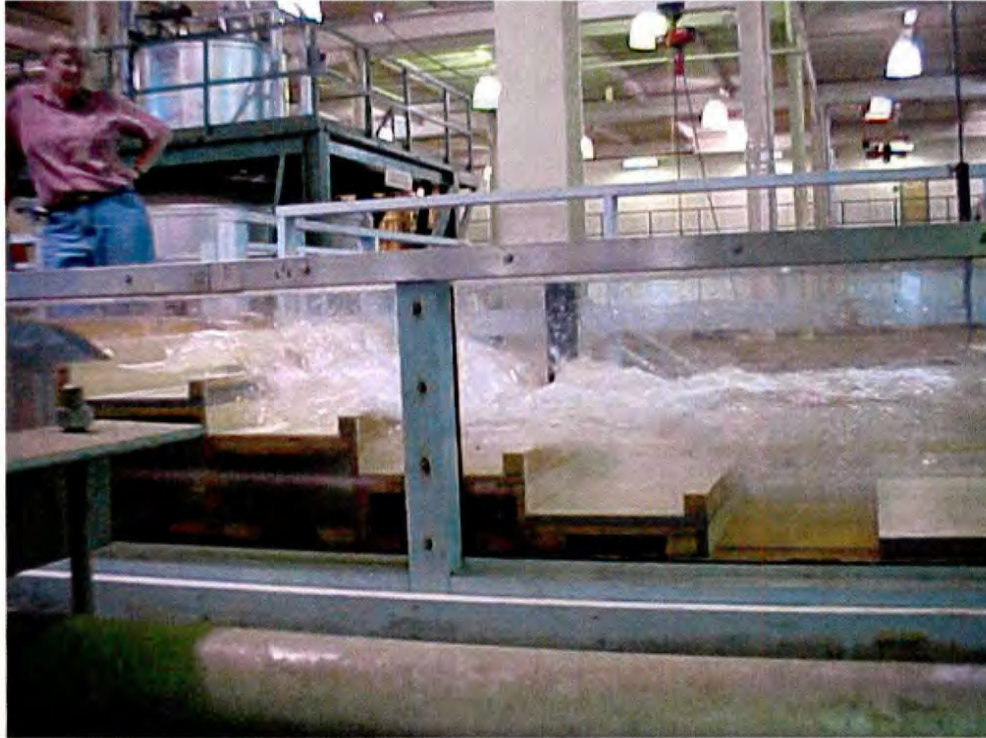
Figure 5: Six foot step length; Q = 330 \text{ ft}^3/\text{s} , TW = 165 \text{ ft}^3/\text{s}
