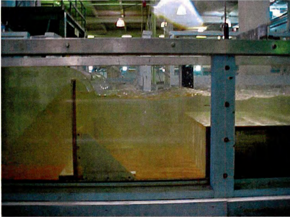
Figure 8: 33 ft. Single Drop with Plunge Pool; Q = 330 \text{ ft}^3/\text{s} , TW = 165 \text{ ft}^3/\text{s}
