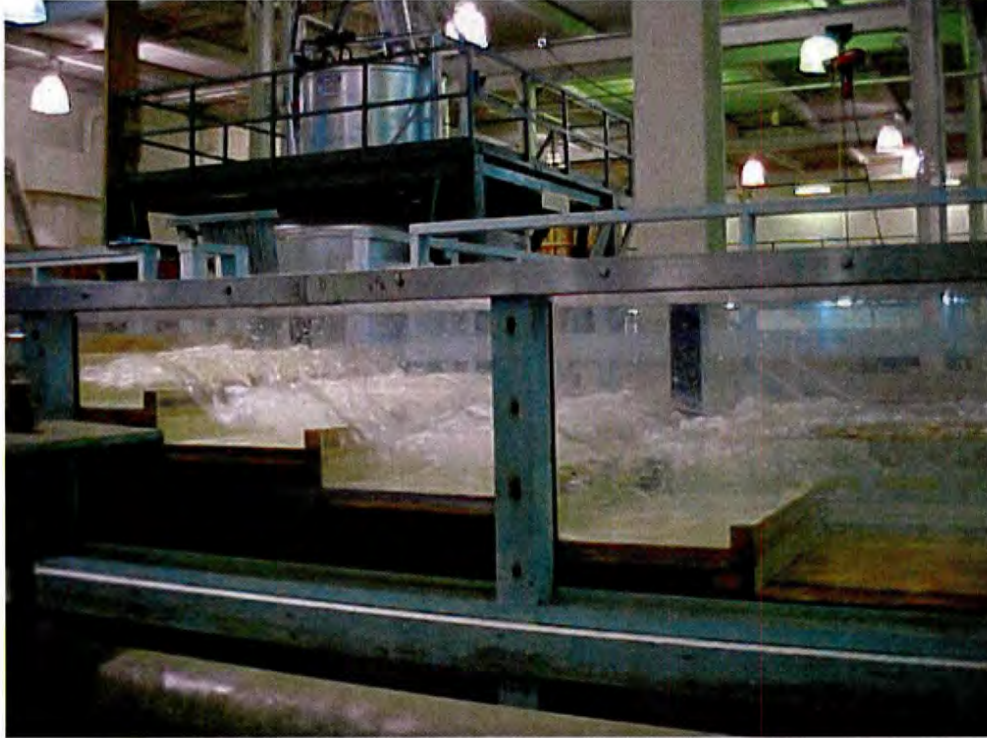
Figure 6: Eight Foot Step Length; Q = 330 \text{ ft}^3/\text{s} , TW = 165 \text{ ft}^3/\text{s}
