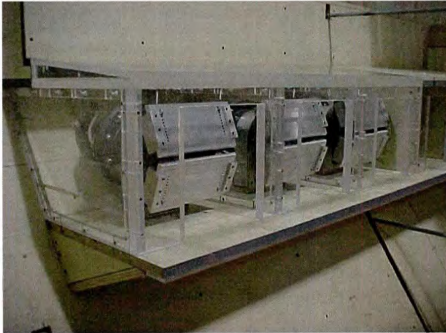
Figure 3 - 1:10 Froude-scale model of three adjacent clamshell gates and appurtenances.
