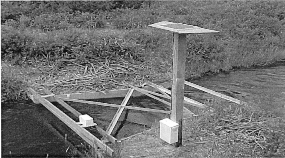
Figure 5. The complete CFM and sensor setup, including solar power. The sensor is mounted on a Parshall Flume under a protective cover.
