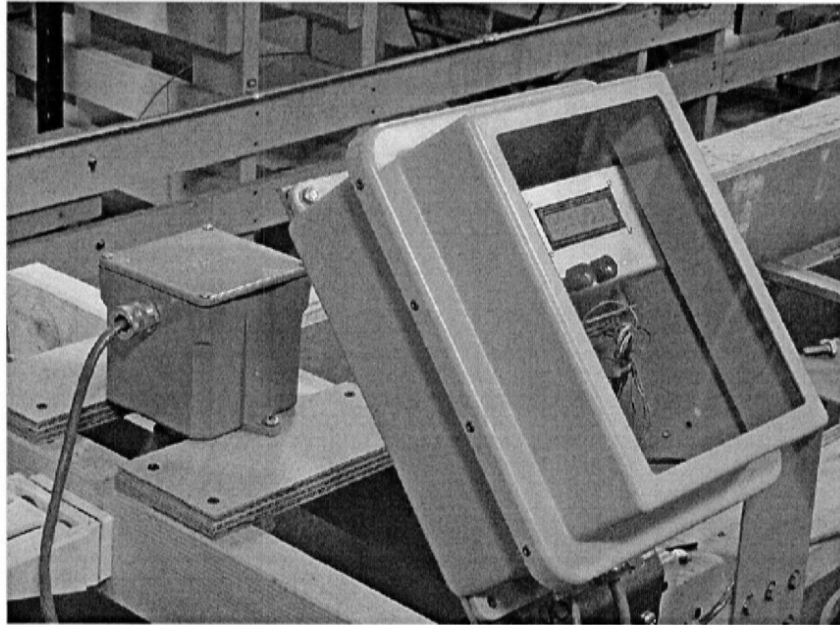
Figure 2. Continuous flow meter mounted in Reclamation's Water Resources Research Laboratory. The ultrasonic sensor is located in the smaller enclosure to the left while the CPU and display are located in the enclosure to the right.
