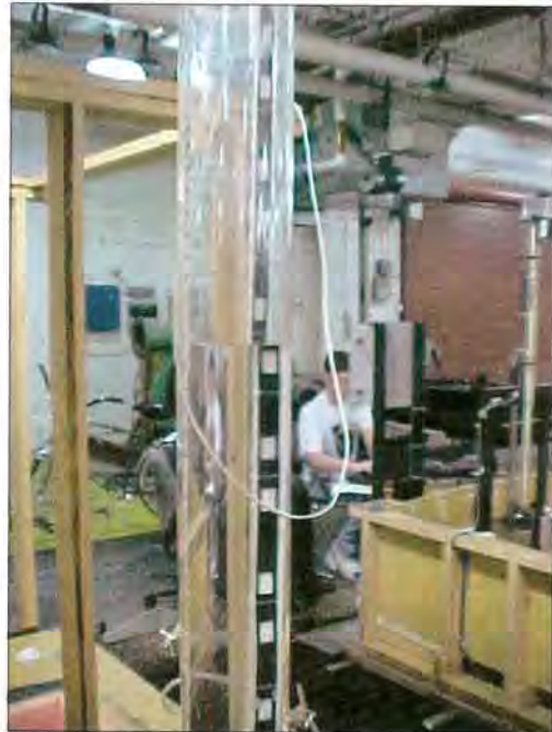
Figure 5. - Laboratory test setup of the high frequency cable water level sensor. In the foreground, the 7-ft-long coaxial cable is mounted in a PVC pipe with a relief valve at the bottom to vary the water level. Data is being recorded by the people in the background where the electronics are located on a table.
