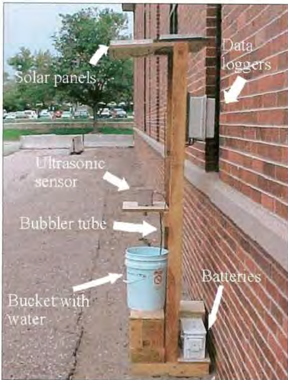
Figure 10. - Long term side-by-side testing of the OCFR and the bubbler system. Both instruments are sensing and recording the water level in the bucket.
