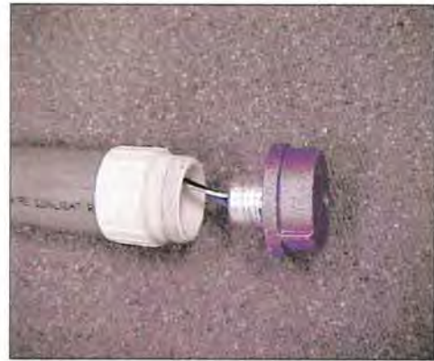
Figure 4. - Pressure transducer threaded into a pipe cap prior to attaching the cap to the end of the PVC tubing. The voltage is then transmitted to a chosen recorder.
