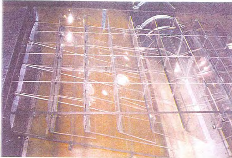
Figure 4. - Photograph #3 - Original baffle configuration.
