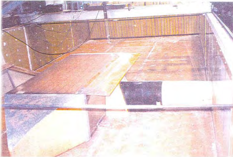
Figure 8. - Photograph #6 - Flow plate modification.
