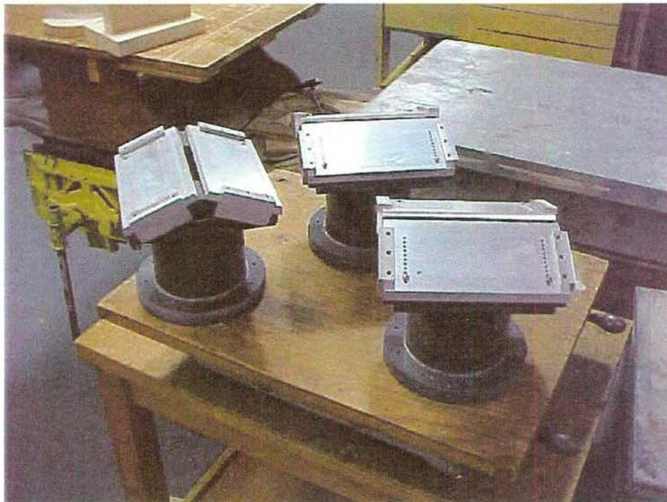
Figure 2. - Photograph of the 4.5-in diameter slide-gate arrangements used to model the 48-in clamshell gates at a 1:10.667 scale.
