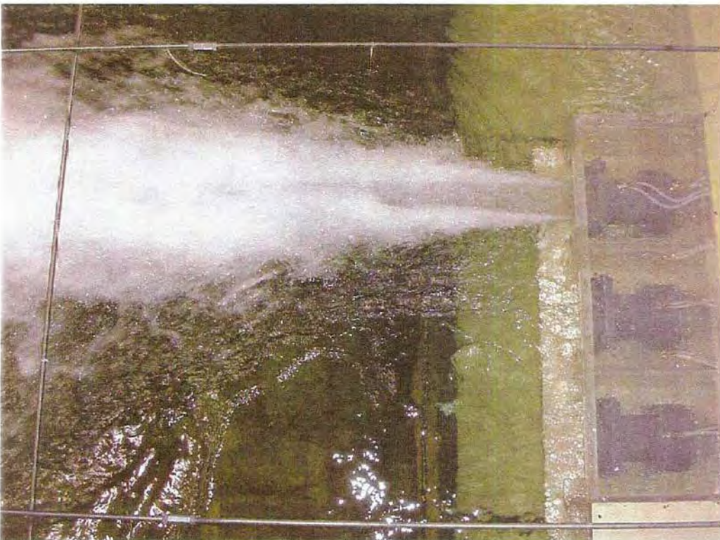
1 gate operated at 100% open under partial submergence.
