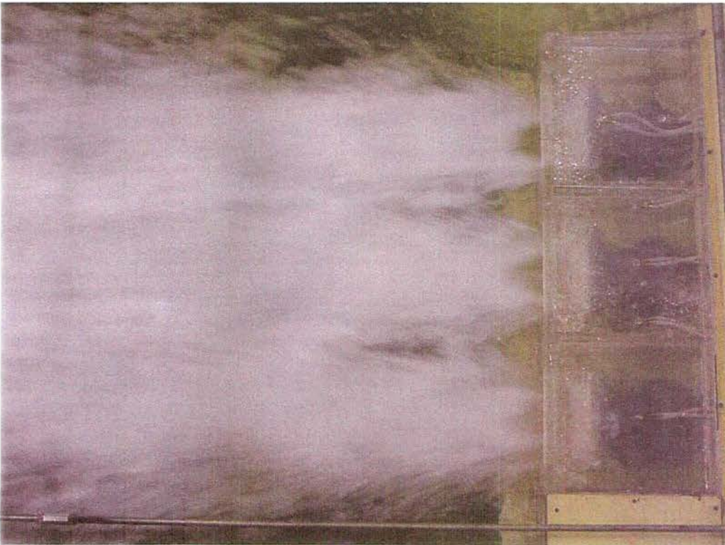
3 gates operated at 10% open under partial submergence.
