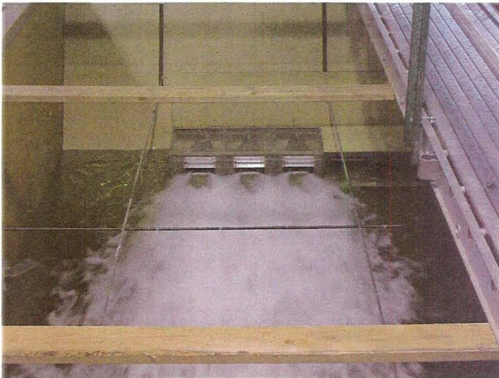
3 gates operated at 50% open under partial submergence.
