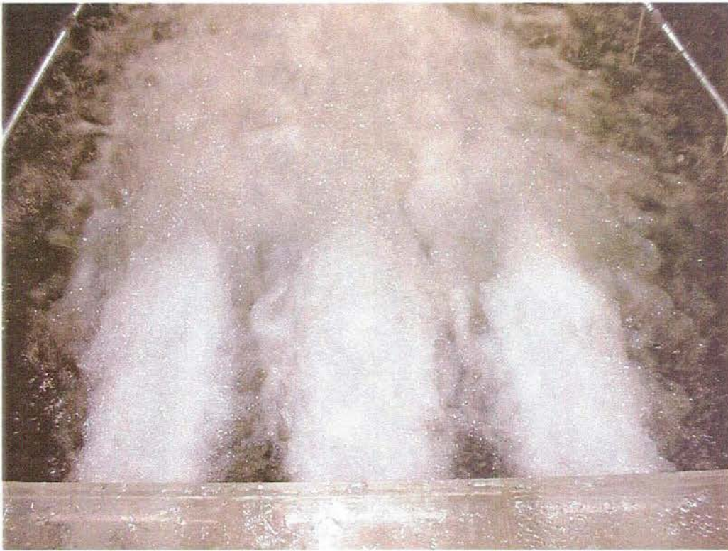
3 gates operated at 10% open under partial submergence.
