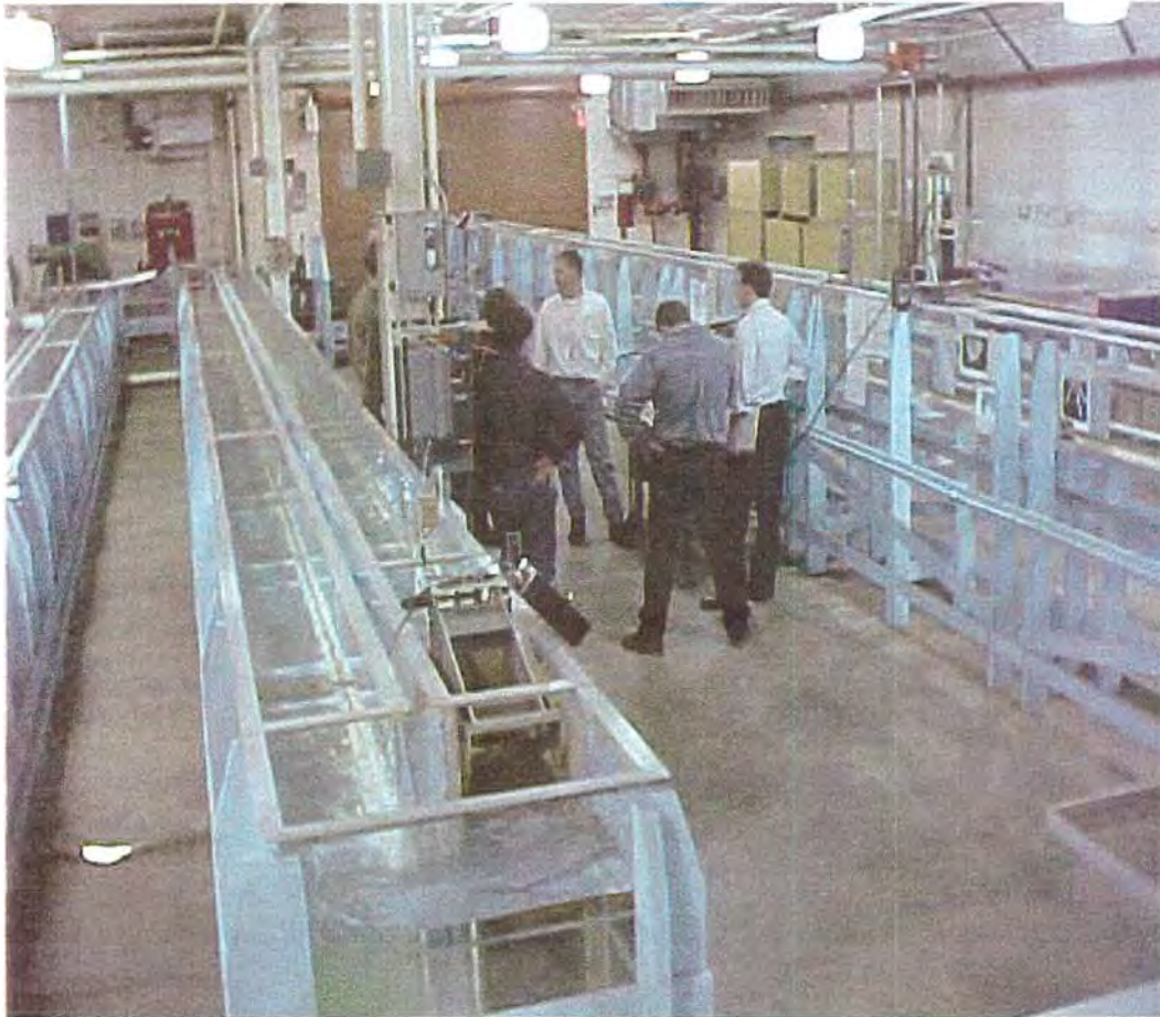
Figure 1 - Canal model in Reclamation's Water Resources Research Laboratory in Denver. The 100-m-long canal is equipped with a variety of gates and instruments. The facility is used for development, demonstration, and training.
