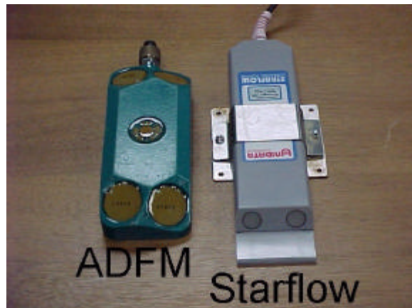
Figure 2. Photograph of the ADFM and Starflow transducers.
