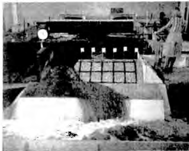
Fig. C-8. Fuse plug test; lateral erosion in progress, initial breach is complete.
