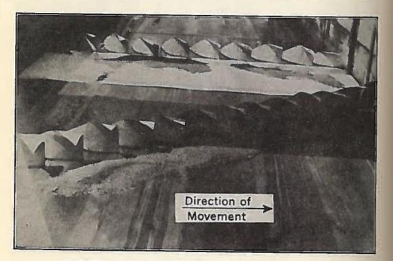
FIG. 3.—EXPERIMENTAL [RIFFLE VANES SET AT ANGLES OF 90° AND 135° WITH THE AXIS OF AN EIGHT-FOOT LABORATORY CHANNEL
