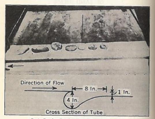
FIG. 1.-FOUR-INCH TUBE SET 90° TO THE AXIS OF THE CHANNEL
