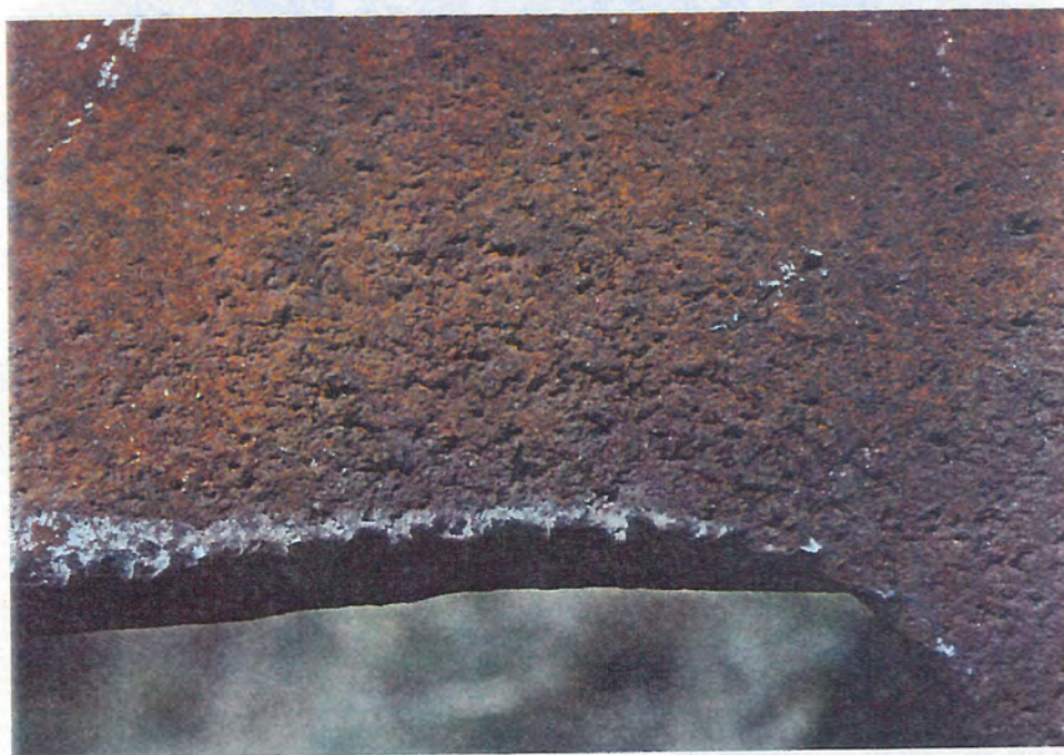
Figure 12. Close-up of Cavitation Damage, Interior Surface
