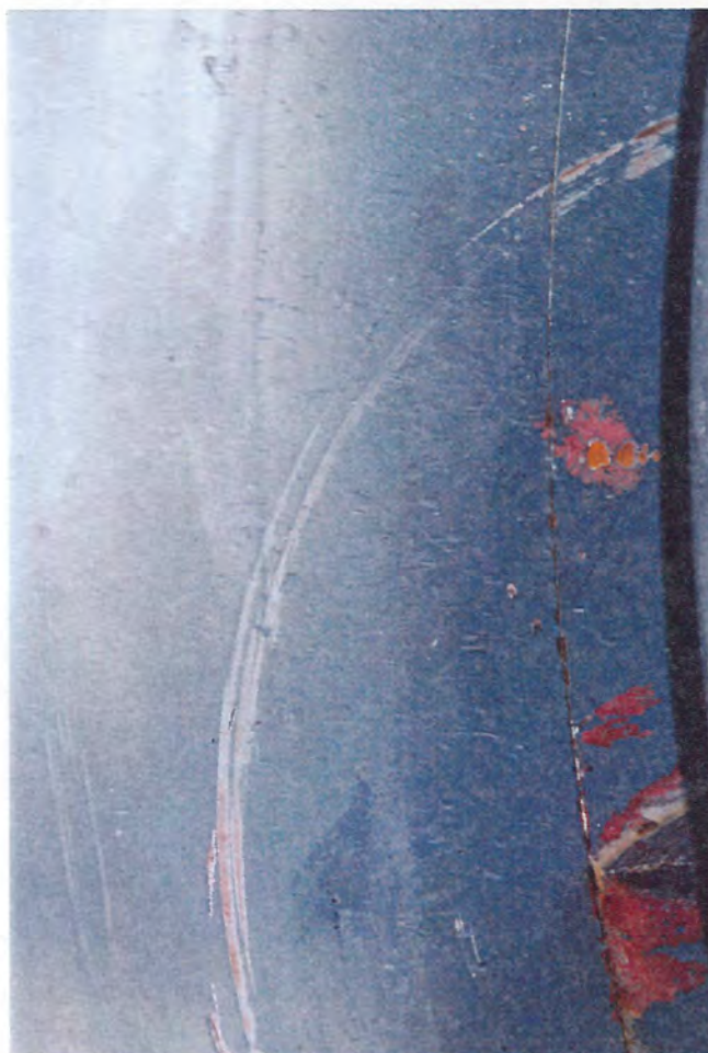
Photograph 10 - Scrape marks where broken piece of outlet pipe traveled through stay vanes of the hollow jet valve.
