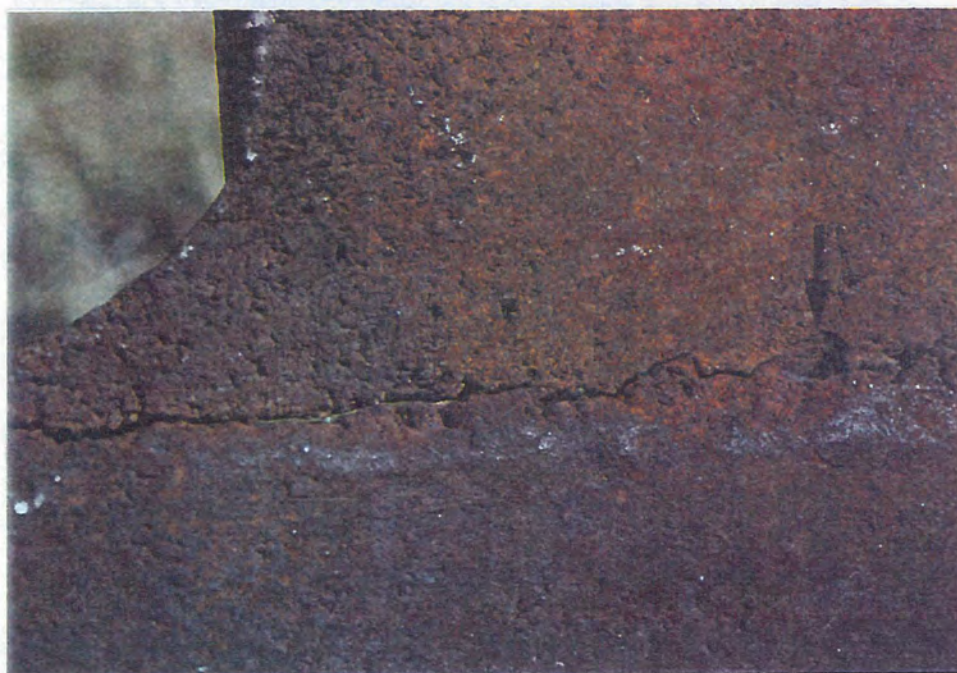
Figure 10. Cavitation Damage and Low Cycle Fatigue
