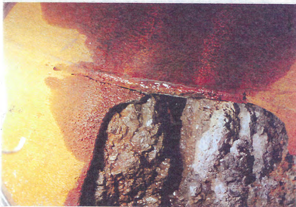
Figure 2. View of Fracture Along Weld
