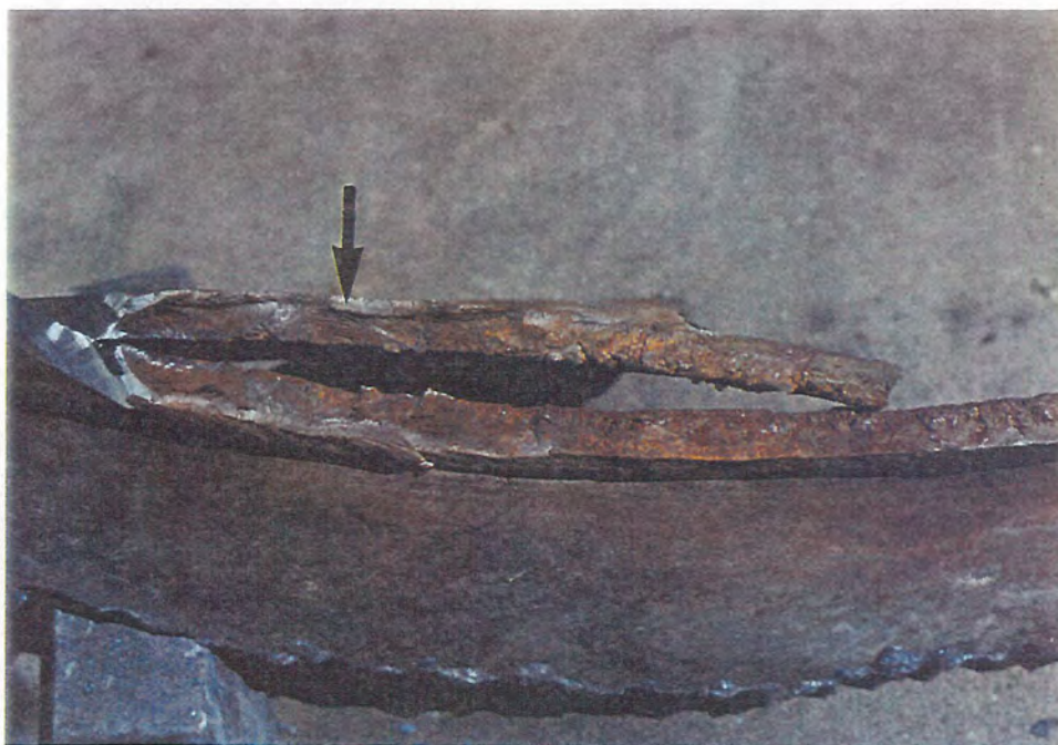
Figure 11. Matching Fracture Surfaces of Crack of Figure 10
