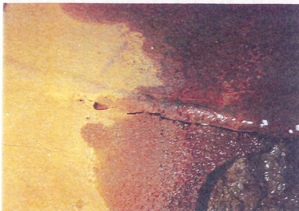
Figure 3. View of Extension of Fracture Adjacent to Piece Torn Out
