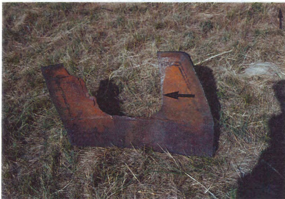
Figure 8. Section Removed From Pipe For Fractographic Examination
