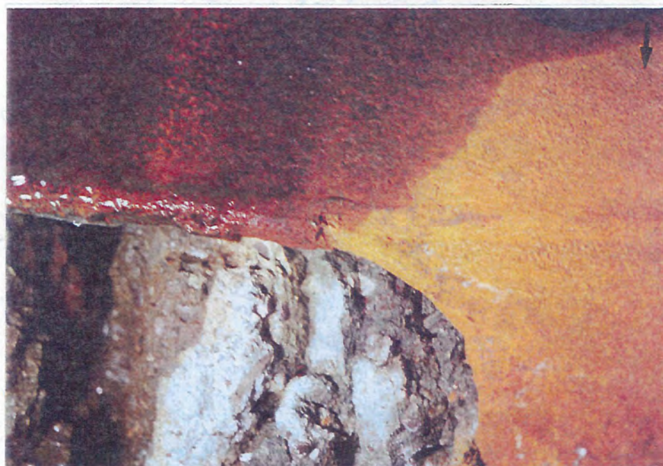
Figure 4. Area Where Fracture Deviates From Heat Affected Zone
