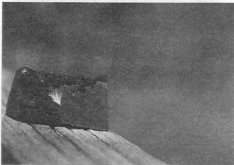
Figure 14. Polished Section Showing Depth of Cavitation Pit
