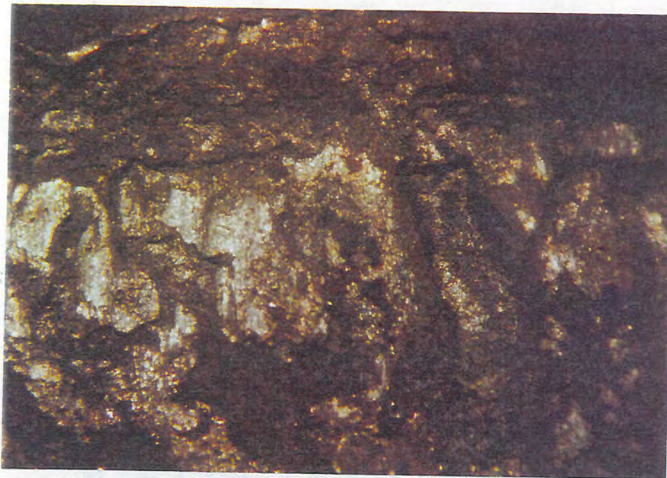
Figure 17. Erosion Through The Plate
