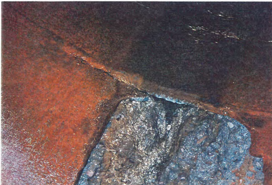
Photograph 7 - Fractured weld. Note crack extends between two large cavitation pits.
