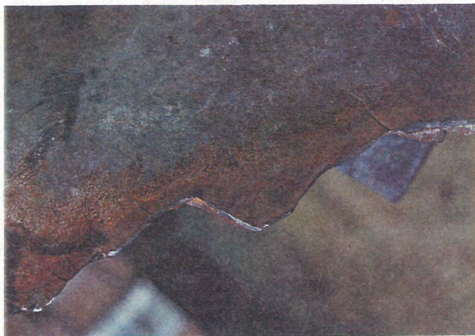
Figure 9. Lateral Cracking Along Fracture Surface
