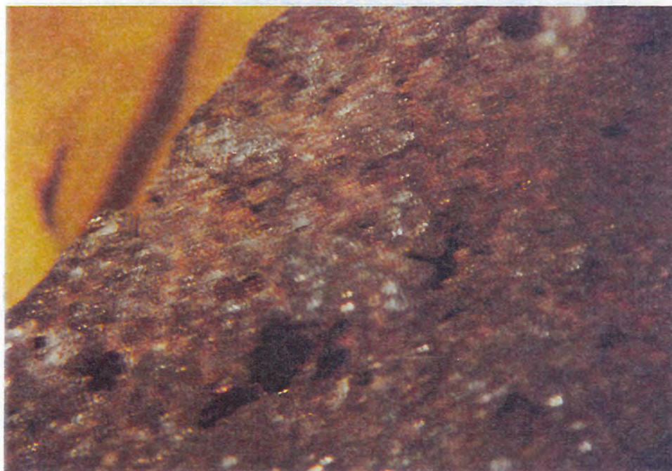
Figure 16. Cavitation Pits As View From Surface
