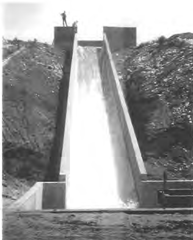
Figure 1. - The Overtopping Facility at CSU is 10 ft wide with a 50-ft drop over a 2:1 slope. Shown is the empty flume with water flowing down the concrete floor of the flume.
