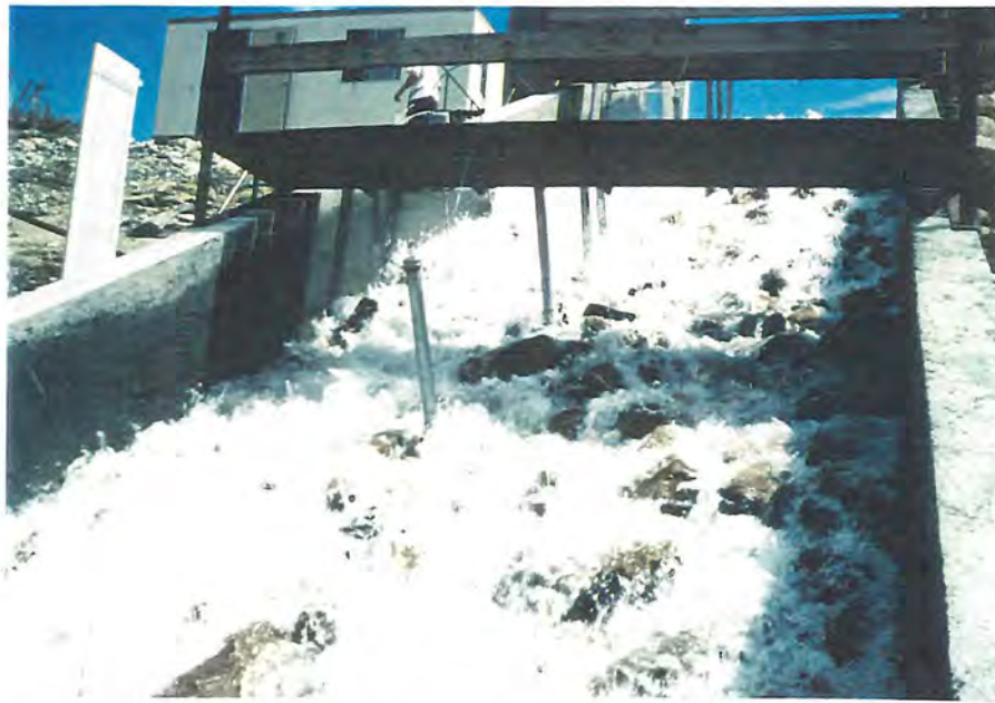
Figure 4. - View looking down onto the surface of the 1994 riprap layer with q=2.0 \text{ ft}^3/\text{s/ft} .
