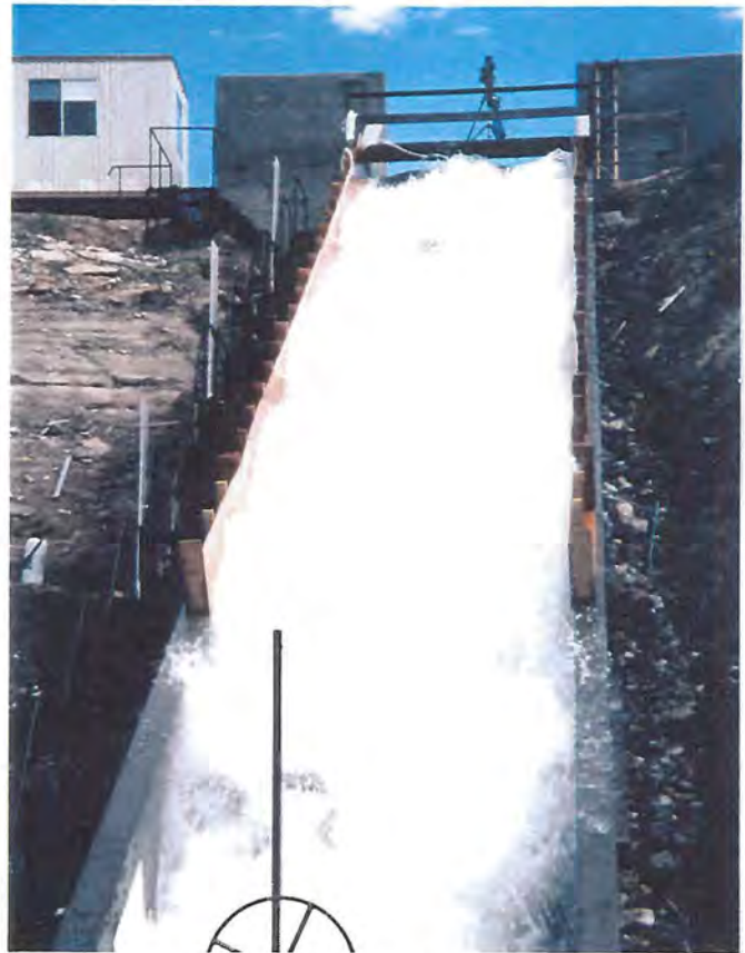
Figure 5. - Overall view of 1995 riprap material with q=8.0 \text{ ft}^3/\text{s/ft} .
