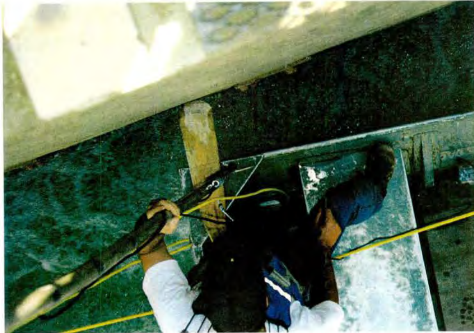
Figure 5. Photograph: Air concentration probe. Setup used for taking air concentration measurements along diffuser wall.
