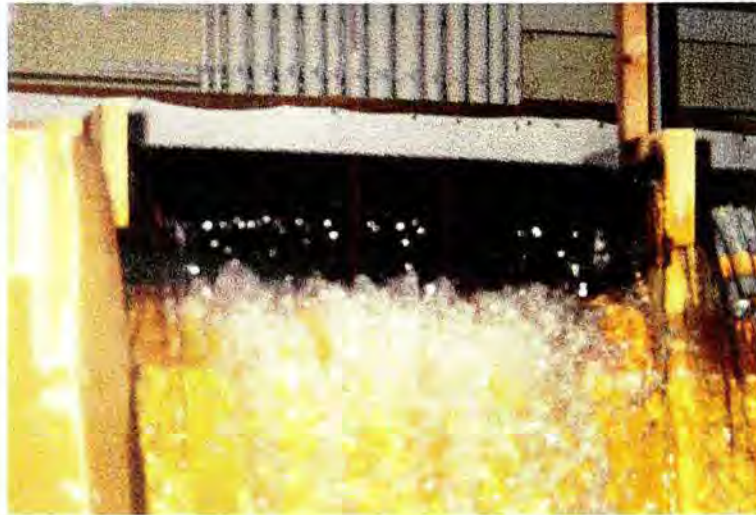
Figure 20. Sumigate model gate #2. This gate performed well with gate heights greater than 12 ft and all overtopping heads. When the gate was nearly deflated, it oscillated due to the end of the gate extending into the negative pressure zone.
