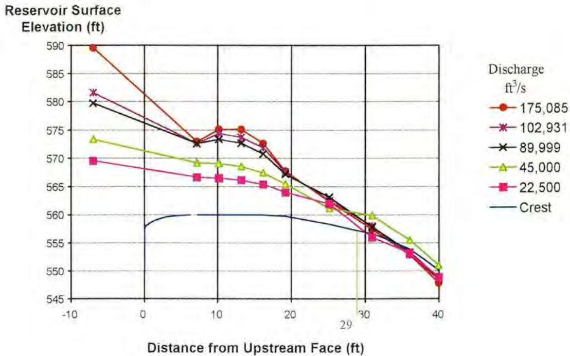
Figure 17. Pressures for the elliptical configuration, measured at the center of the spillway bay. The maximum rubber gate layout length for this section is 23 ft.
