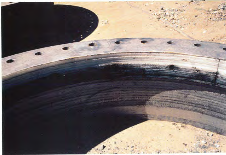
Figure 8: Damaged UHMW wearing ring and packing from Archimedes pump.
