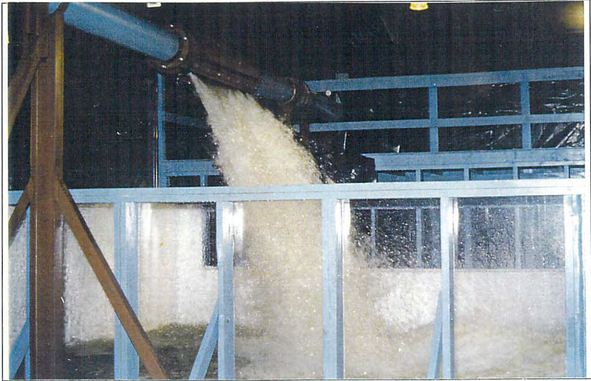
Figure 4.7 Dam overtopping model in operation
