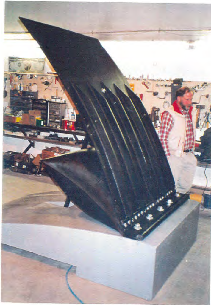
Photograph 7 - A Fort Collins, Colorado, company manufactures a gate that is raised and lowered by an air bladder.
