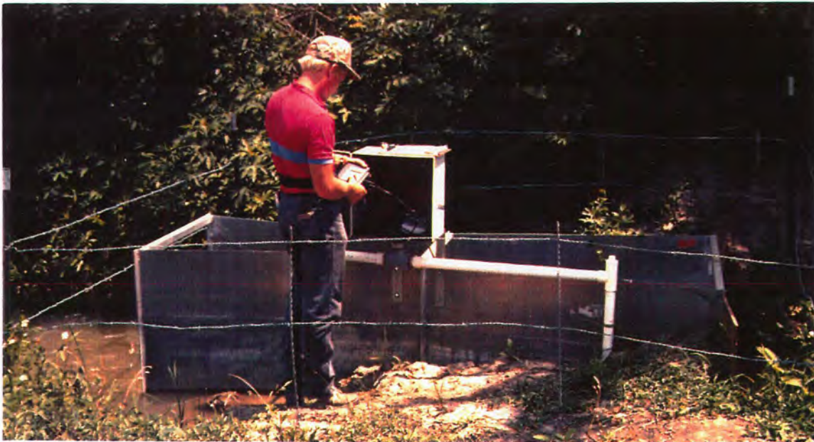
A LCRA employee recording flow data at a Parshall flume.
