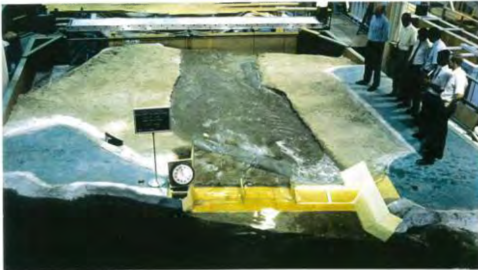
Figure 3. - Flow of 4250 m 3 /s through the first two sections of the Horseshoe Dam Fuse Plug Model. Scale 1:60.
