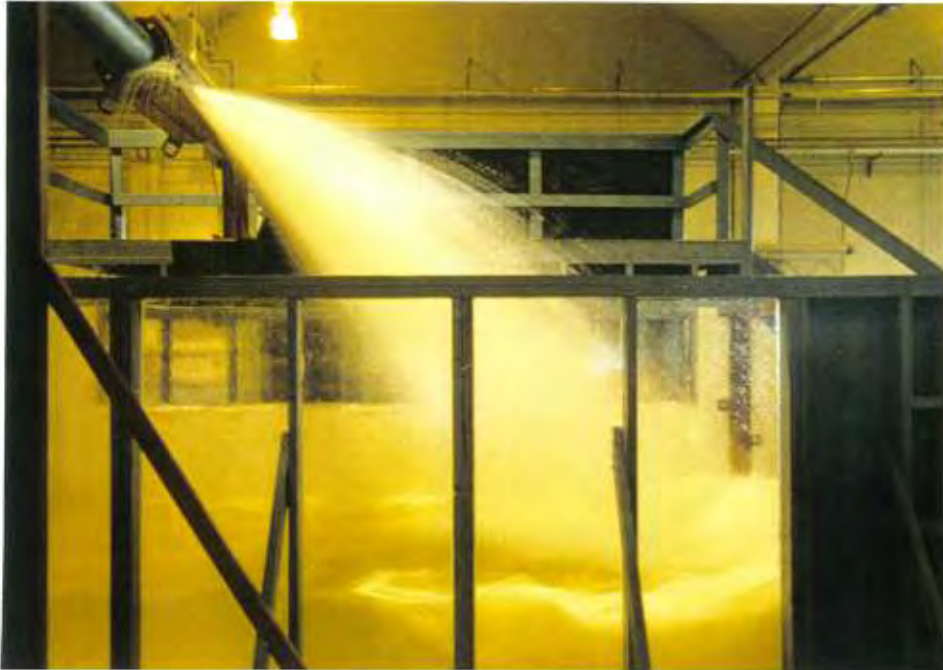
Figure 5. - View of 1:3 scale laboratory model with orifice jet discharging into basin.
