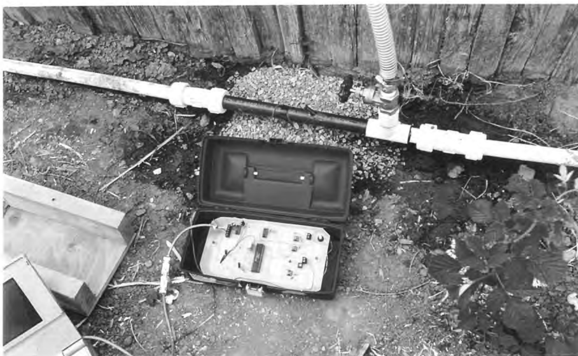
Figure 10. Meter pipe insert and strain gauge field installation.
