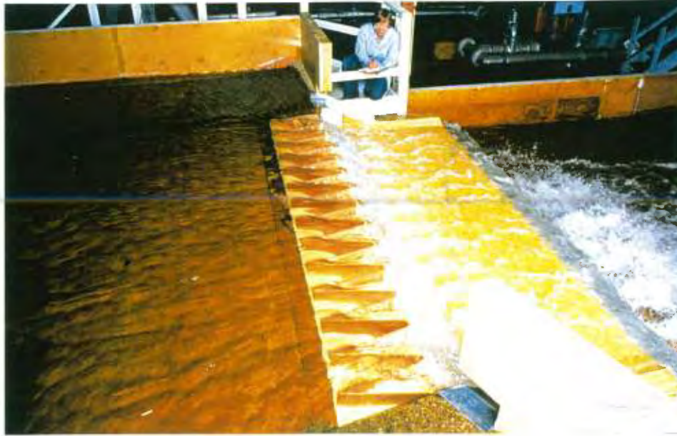
Figure 1. - View of the 1:80 scale model of the 14-cycle, 9-m-high Ute Dam labyrinth crest passing 15 500 m 3 /s.
