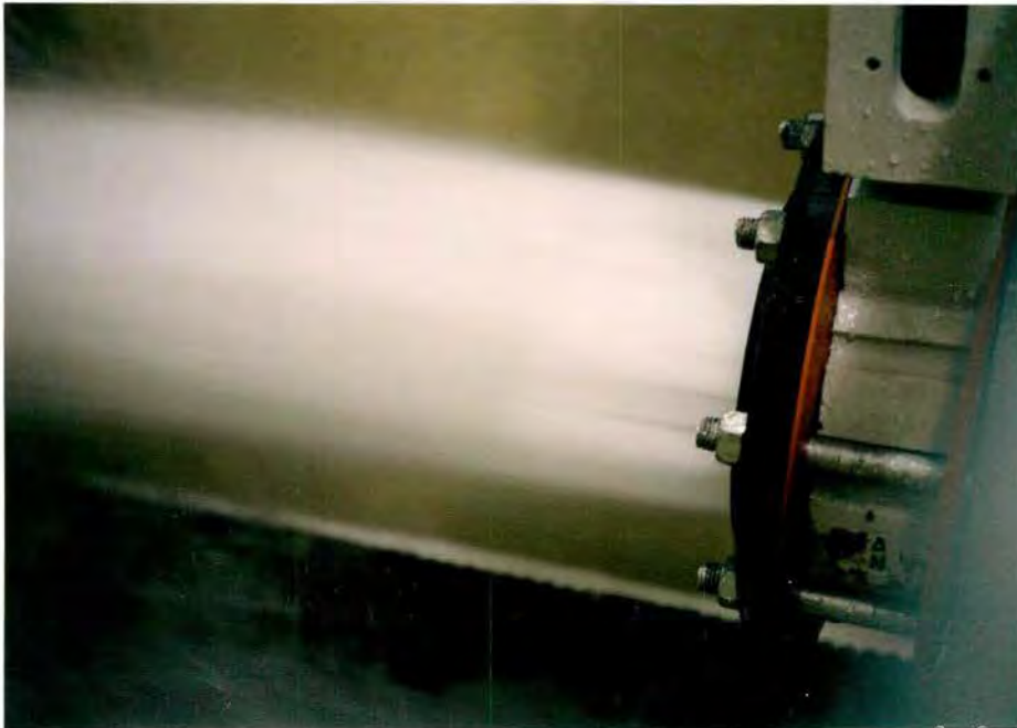
Figure 10b: 8-inch Monovar, end-of-line discharge, 100-percent open, H=250 ft, note that you can still see individual jets near the valve face.
