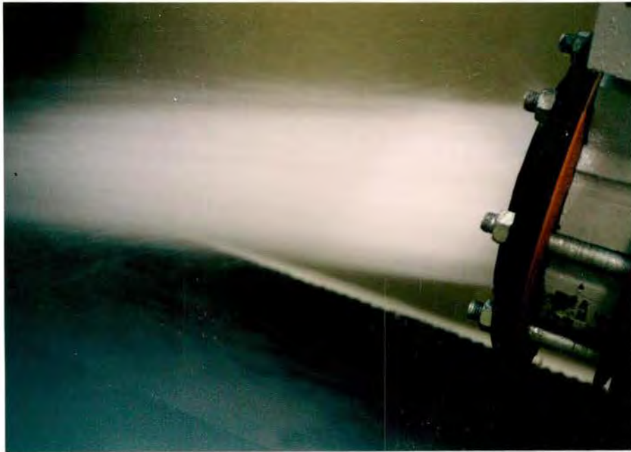
Figure 10a: 8-inch Monovar, end-of-line discharge, 20-percent open, H=250 ft, note downward trajectory of the combined jets.
