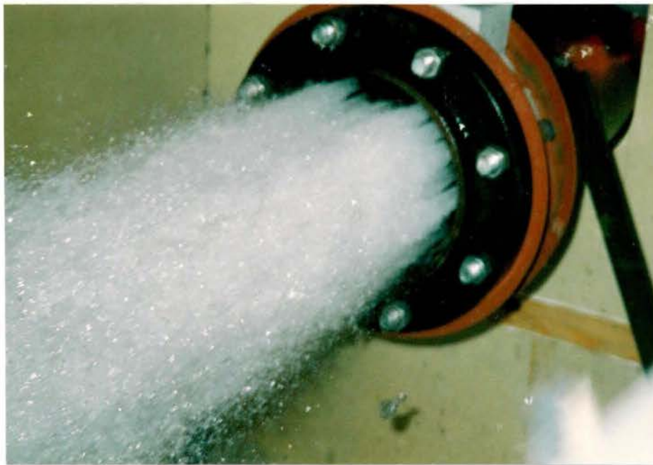
Figure 9b: 8-inch Monovar, end-of-line discharge, 100-percent open, H=50 ft.
