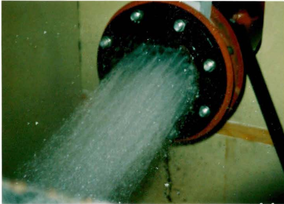
Figure 9a: 8-inch Monovar, end-of-line discharge, 20-percent open, H=50 ft.
