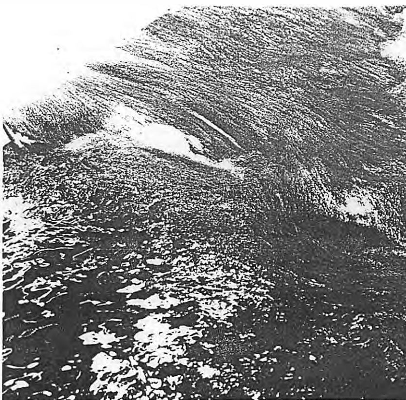
Figure 10. - Flow conditions through channel C, Q = 22,500 \text{ ft}^3/\text{s} with no powerplant flow.
