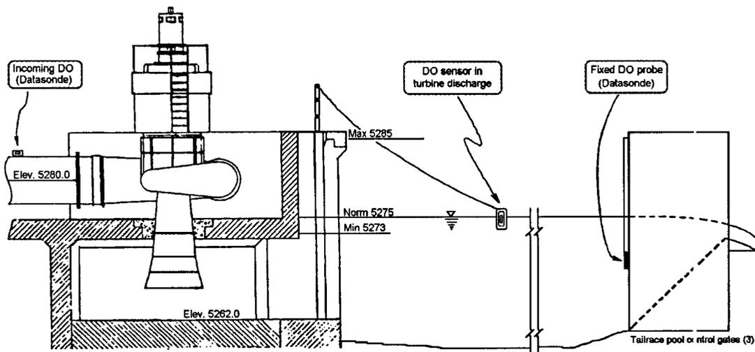
Figure 1. - Deer Creek Powerplant. The turbines installed in 1958 have simple conical diffuser draft tubes rather than formed elbow-type draft tubes for which most turbine aeration research has been done. DO measurements were taken upstream and downstream of the turbines, at the downstream end of the tailrace pool (about 200 ft downstream of the powerplant), and at several downriver locations.
