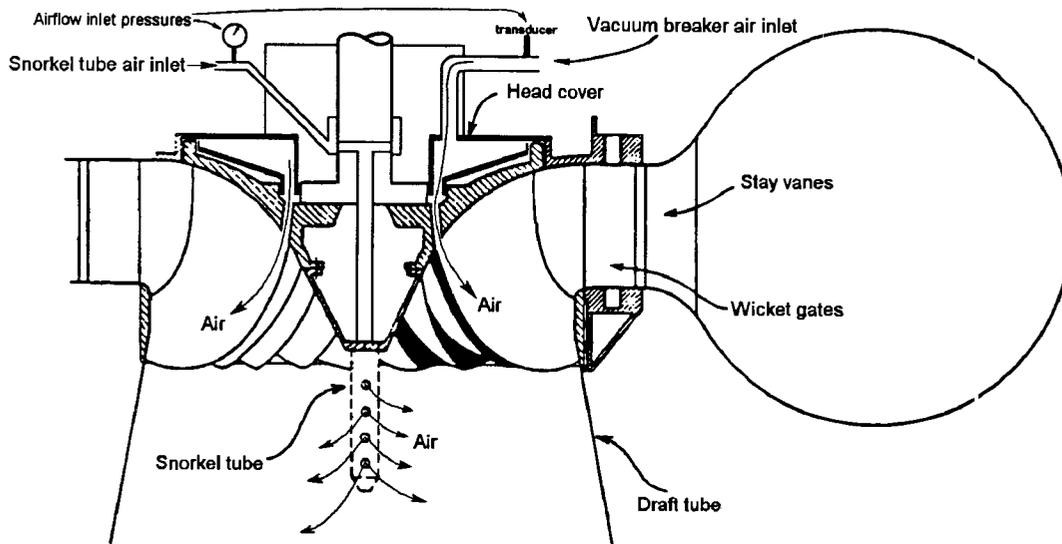
Figure 2. - Air was supplied to the draft tube through the vacuum breaker system (air flows under the headcover and through existing holes in the runner crown) and through the snorkel tube (air flows through a passageway in the shaft).
