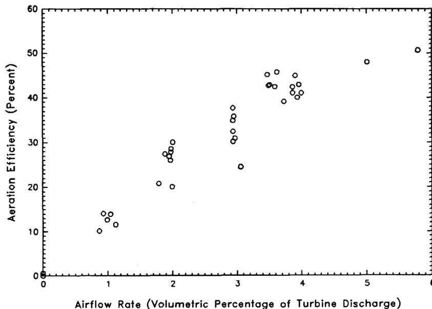
Figure 3. - Aeration efficiency achieved by turbine aeration as a function of airflow rate. This figure includes data collected in the outflow from each turbine, and in the combined powerplant flow at the downstream end of the tailrace pool (recorded with the roving multi-parameter probes). It does not include data from the Datasonde installed in the pipe at the end of the tailrace pool.
