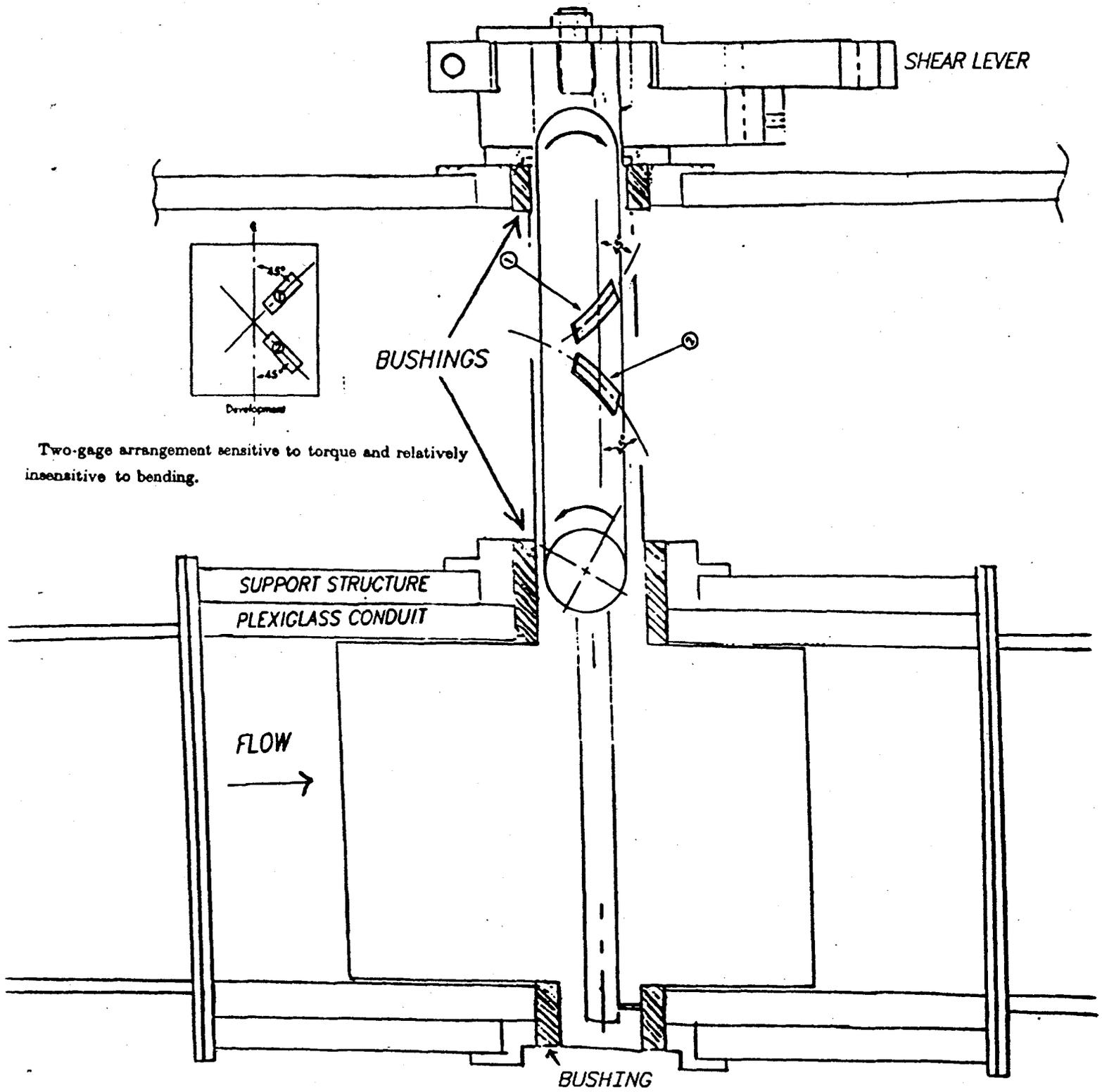
Two-gage arrangement sensitive to torque and relatively insensitive to bending.
