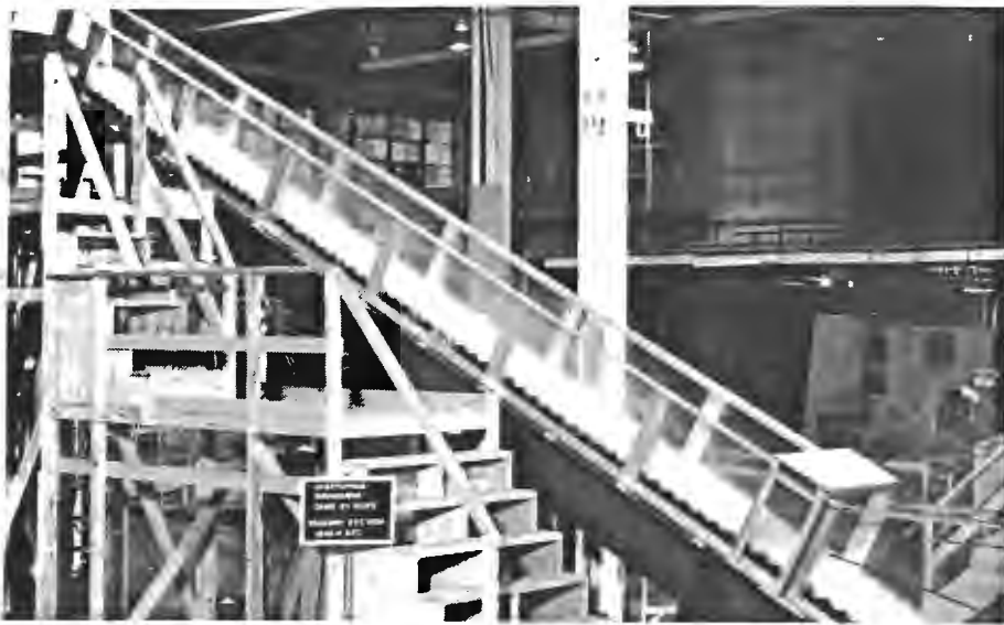
Reclamation's newest laboratory flume facility is being used to develop design criteria for stepped forms of overtopping protection for high embankment dams. The flume is 1.5 feet wide, has Plexiglas walls, and has a variable slope with 15.5 feet of vertical drop. This photograph shows the flume set at a 2:1 slope with a unit discharge of 1.16 ft 2 /s and 0.42 feet of overtopping head.
