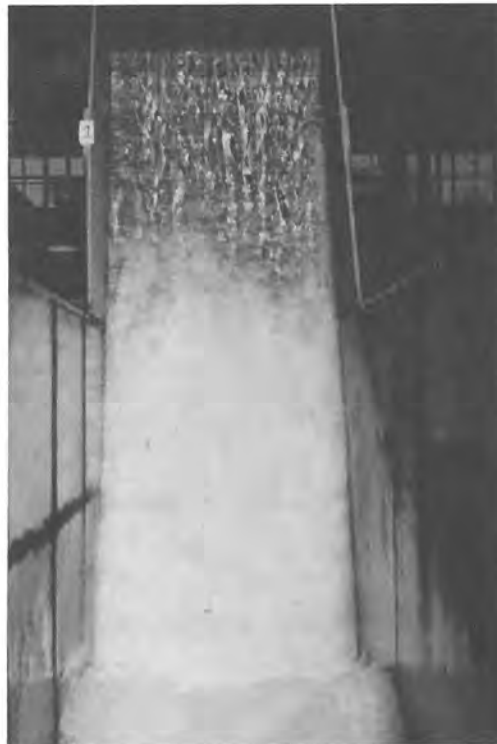
Figure 11. - 11.6 \text{ m}^3/\text{s}/\text{m} unit discharge on the 1:15 scale model of Upper Stillwater spillway (Houston 1987). 1 \text{ m}^3/\text{s}/\text{m} = 10.8 \text{ ft}^3/\text{s}/\text{ft} .
