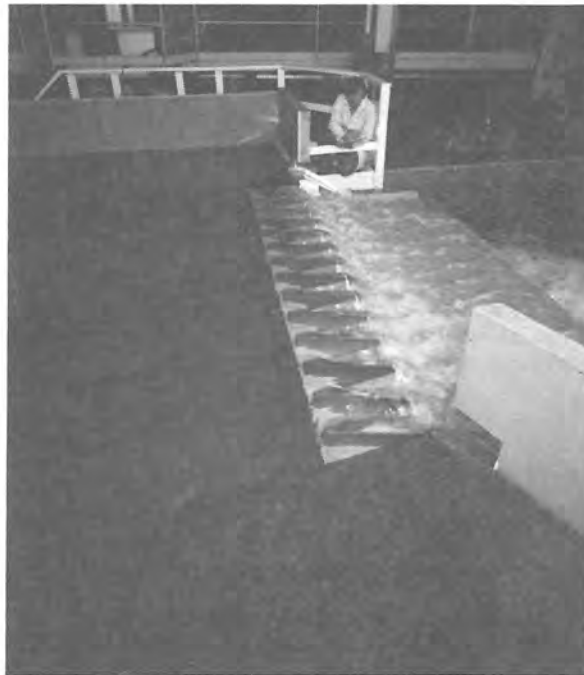
Figure 3. - 1:80 scale model of Ute Dam labyrinth spillway (Houston 1982).
