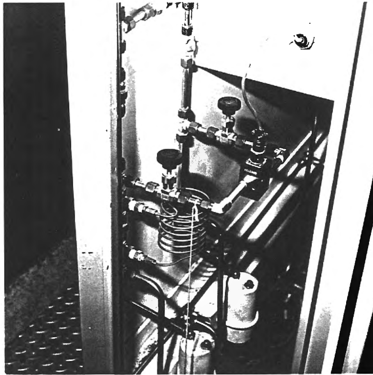
Figure 12: Pressure transducer used as input to PID controller.
