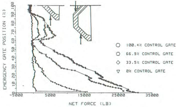
Figure 4. - Force on the emergency gate leaf - unbalanced head operation.
