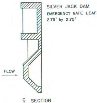
Figure 1. - Section of the gate leaf at Silver Jack Dam.
