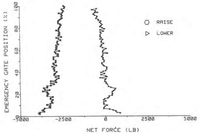
Figure 3. - Forces on the emergency gate - balanced head conditions. A positive net force is in the downward direction.
