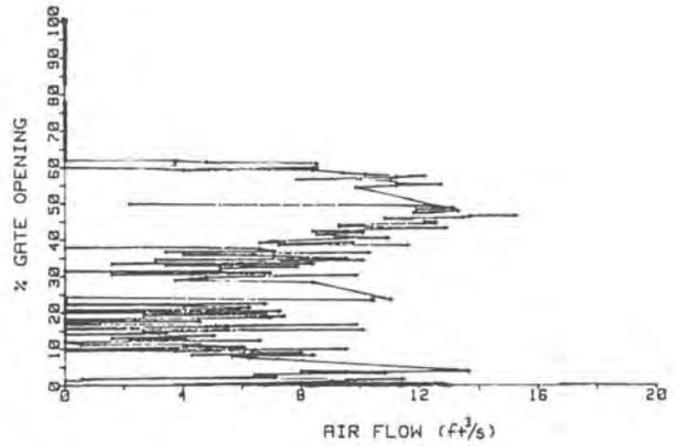
Figure 6. - Air demand at a 100 percent unbalanced head condition.
