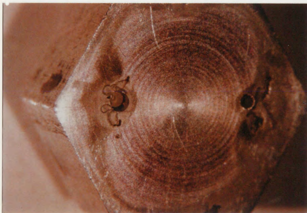
Fig-26. Microscope Photo of Cavitation Pattern on Aluminum Button
