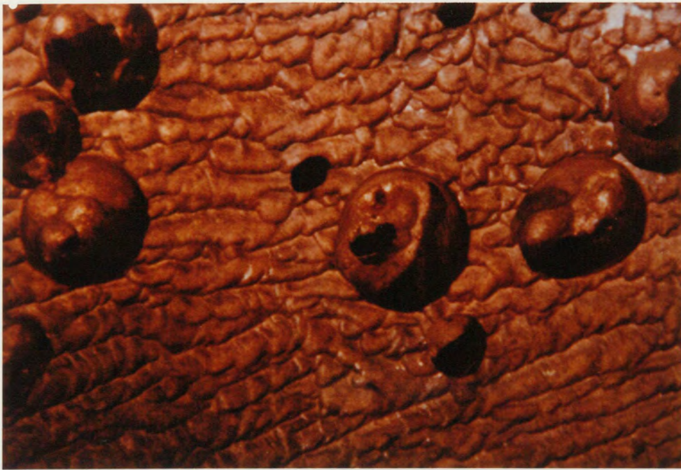
Fig-27. Microscope Photo of Cavitation Damage on Runner of Flatiron Unit 1.
