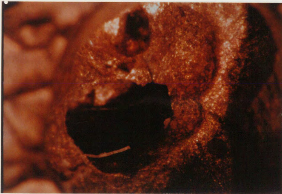
Fig-28. Microscope Photo of Cavitation Damage on Runner of Flatiron Unit 1.
