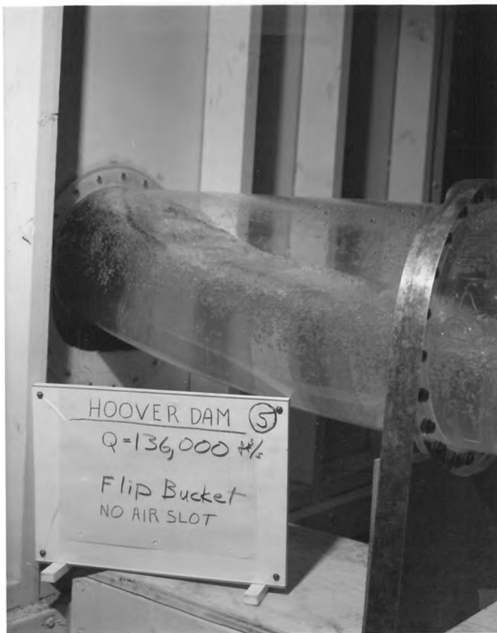
7a Flip bucket at the spillway tunnel exit discharging 135,000 ft 3 /s with a free flow surface
