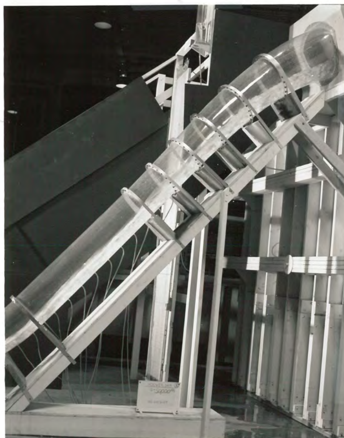
Figure 4.- Flow through the tunnel without an aerator
