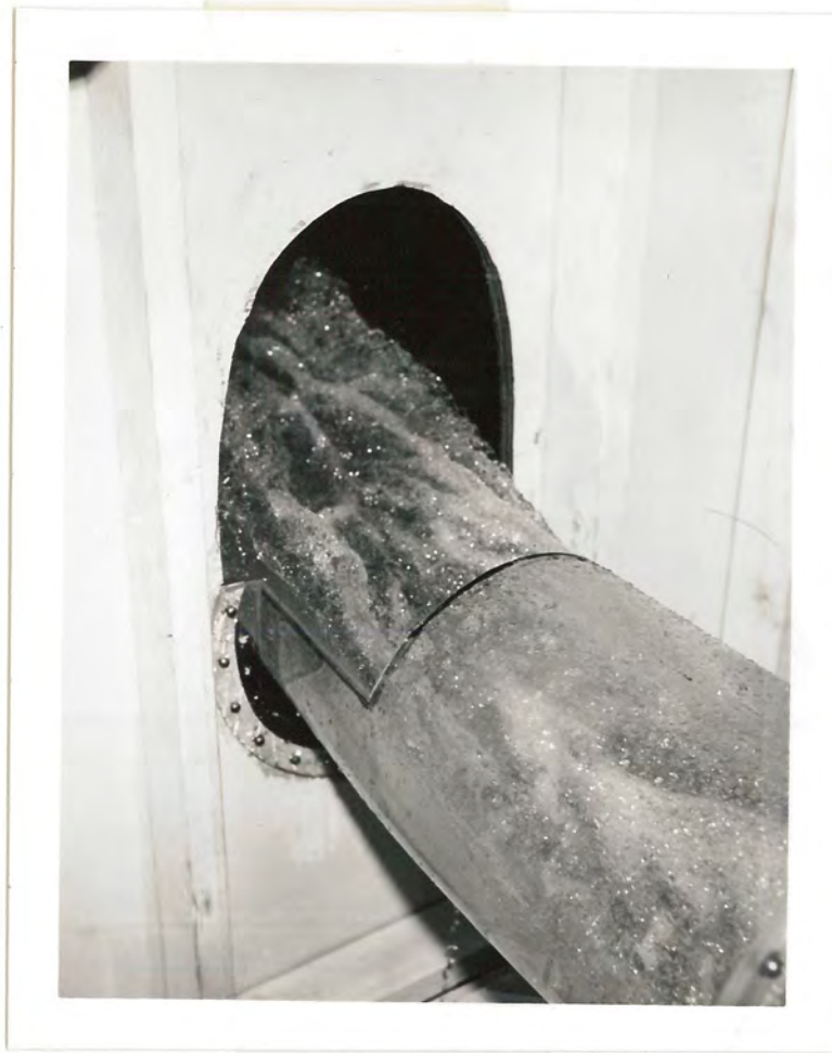
Figure 23 22 — Modified flip bucket passing a discharge of 200,000 ft 3 /s.
