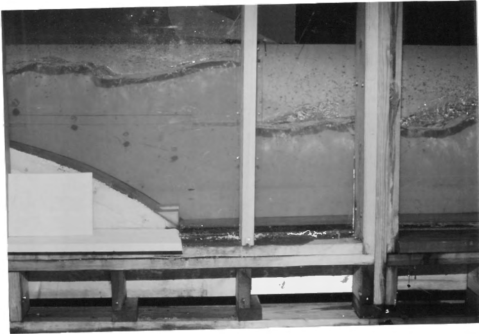
Figure 5. - Sluiceway operation at 4,200 ft 3 /s with the second gate structure downstream of the original slide gates - note the turbulent water surface
