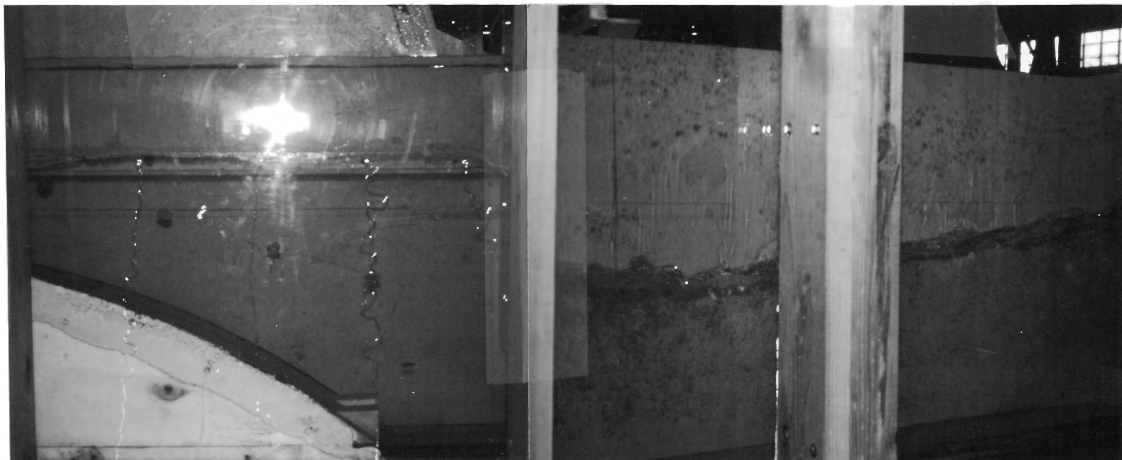
Figure 6. - Sluiceway operation at 4,200 ft 3 /s with the area between the two gate structures covered
