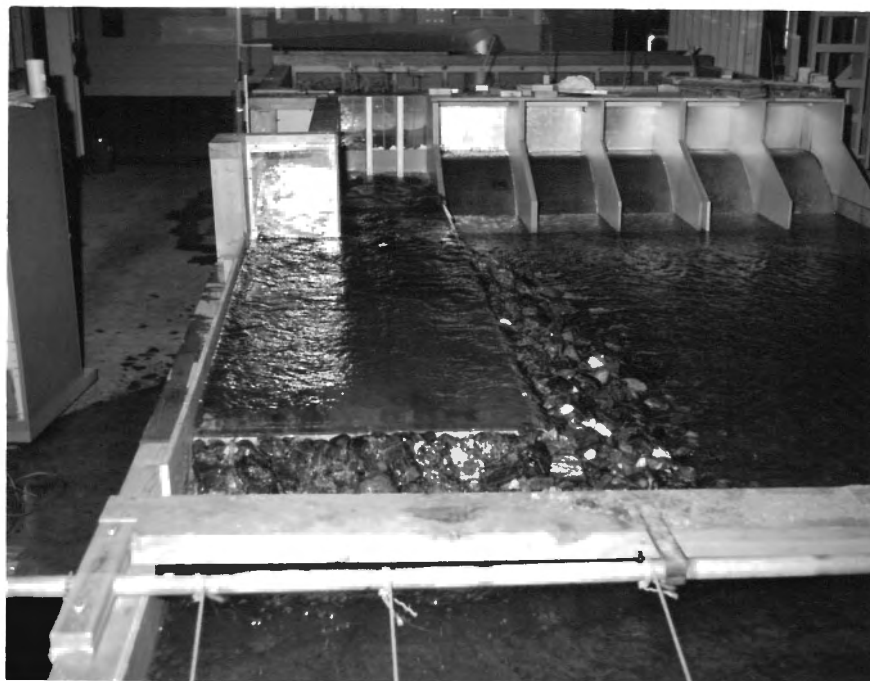
Figure 3. - The cascade at crest elevation 3171, downstream of the sluiceway passing 4,200 \text{ ft}^3/\text{s}
