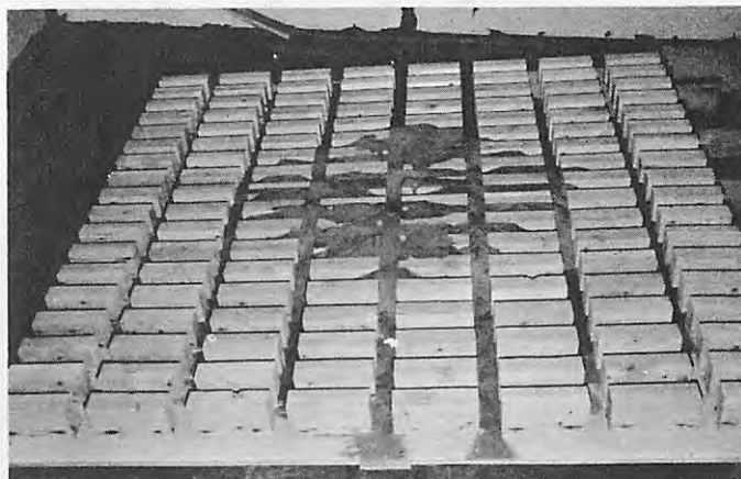
Figure 10. Test 5. This test was a continuation of test 4 in which the backfill deposit was allowed to continue. Mine submerged and dipping 5°. (Distorted model scale)
