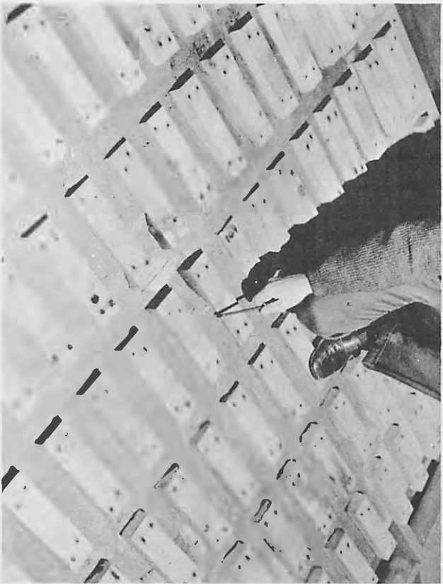
Figure 30. Test 14. Deposit around the injection hole is uniform in a dry cavity with a level floor.
