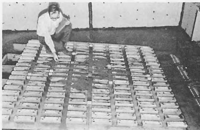
Figure 17. Test 11. Corridor 8 is pointed out in which the total injection flow was concentrated after backfill material filled to the roof around the injection hole. Mine submerged and dipping 5°. Last test in series of three tests, 9-11.
