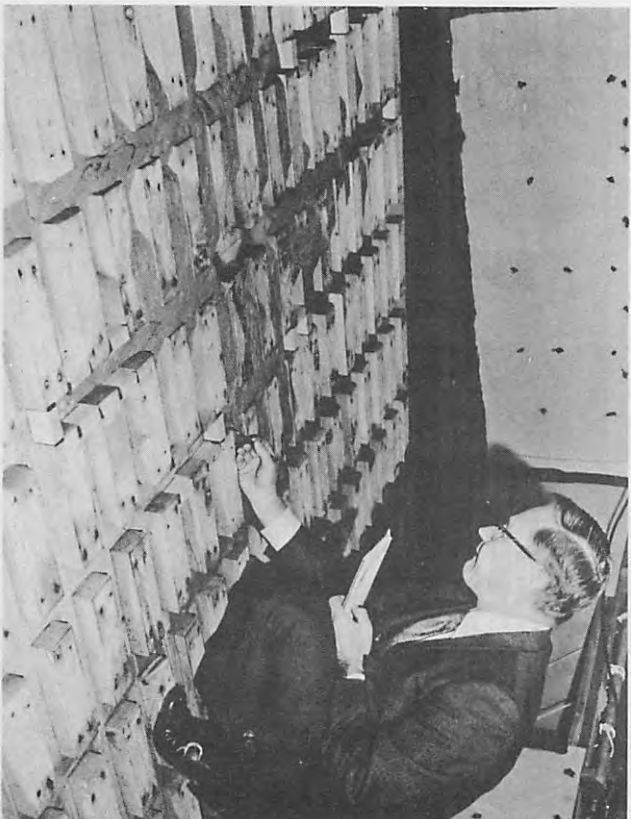
Figure 15. Test 9. First test in the series of three tests, 9-11. Blind entries were simulated by blocking corridors at various places. Mine submerged and dipping 5°.
