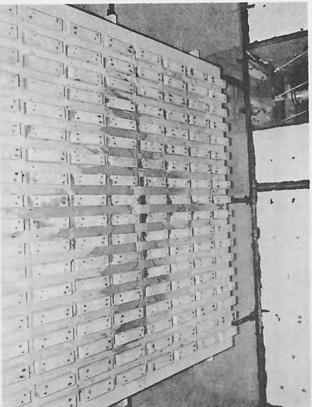
Figure 26. Test 12. The low height of deposit is a result of injection into a dry cavity with a level floor.
