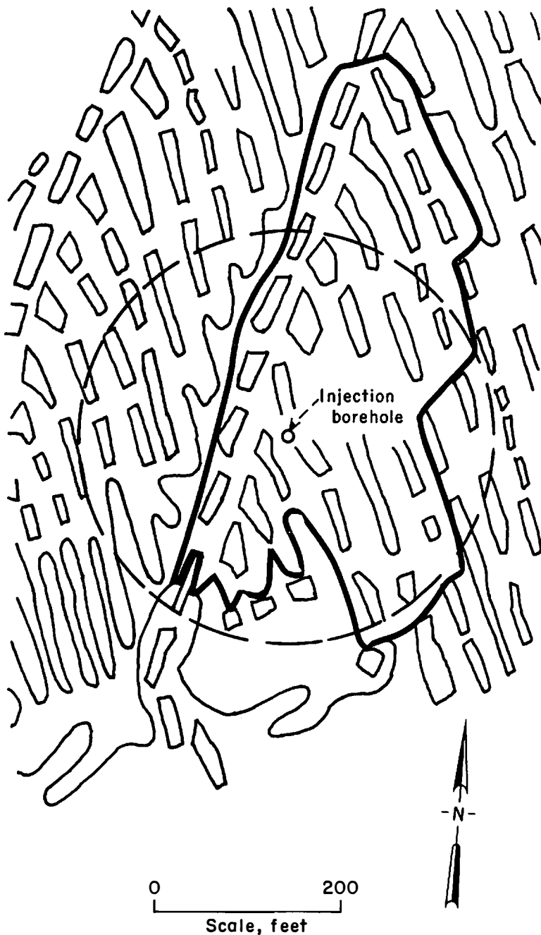
FIGURE 10. - Map of mine workings at the site of the first demonstration project in Rock Springs, Wyo., showing pattern of sand deposition in the mine voids. Dashed circle shows area of planned backfill.
