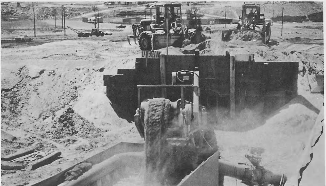
FIGURE 25. - Photograph of sand being bulldozed into hopper and fed from conveyor into mixing tank. (Note jet action at side of tank creating turbulence.)
