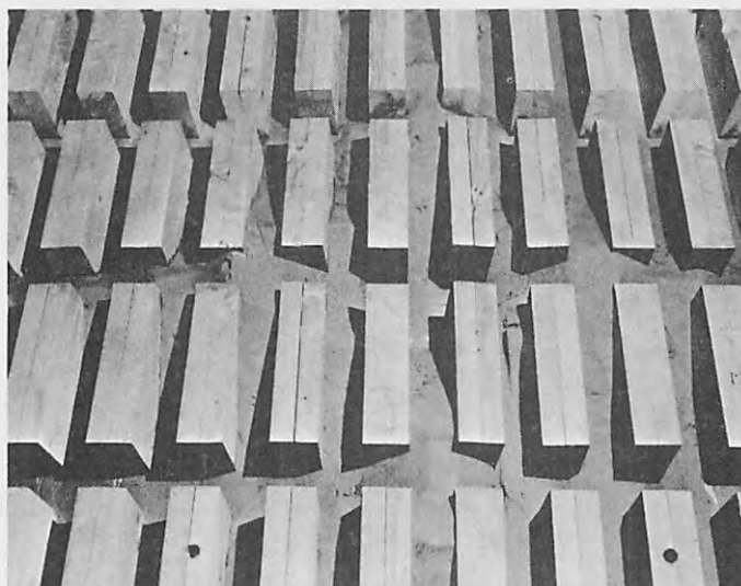
Figure 8. Test 4. The position of the pump intake was changed before test started, causing only a small deposit in the mine cavity during the test. Mine submerged and dipping 5°. (Distorted model scale)
