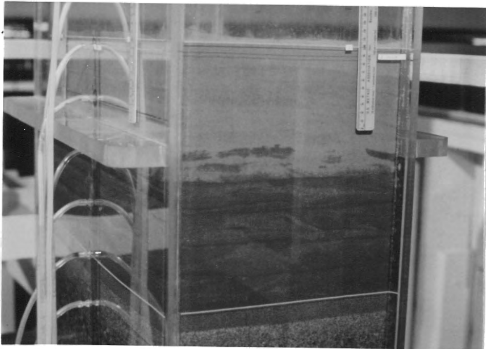
b. Filling sand test specimen box with water, note piezometer taps on front face of the plastic box.
