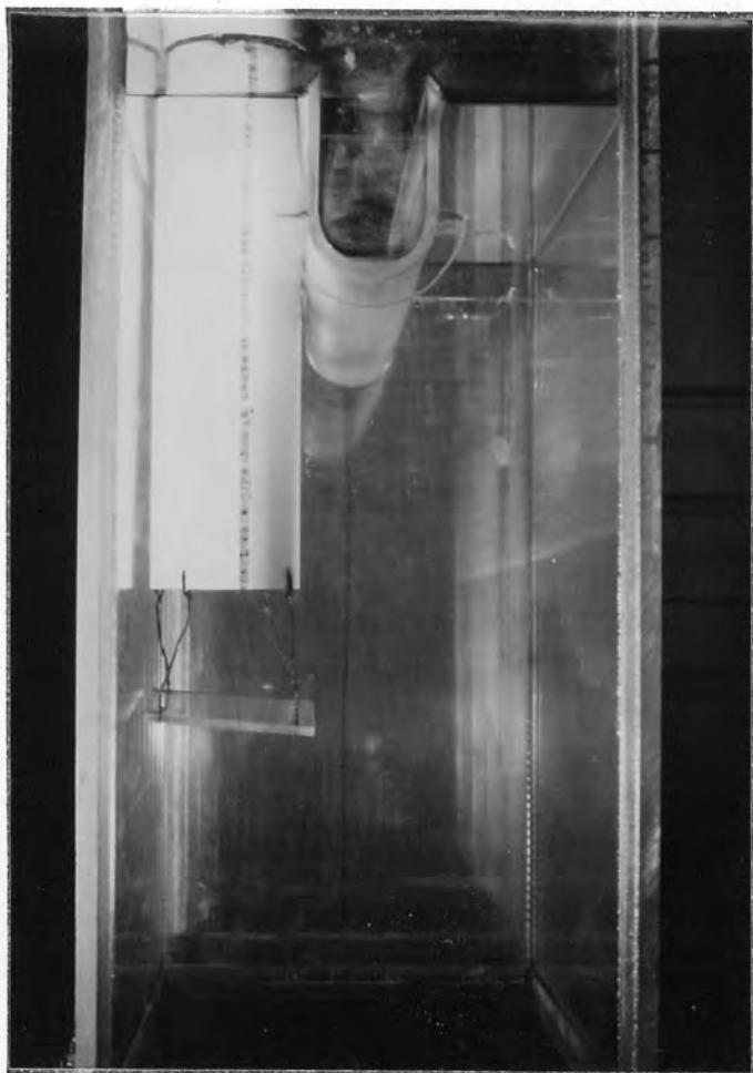
Fig. 1a. Inlet pipe with flow deflector.
