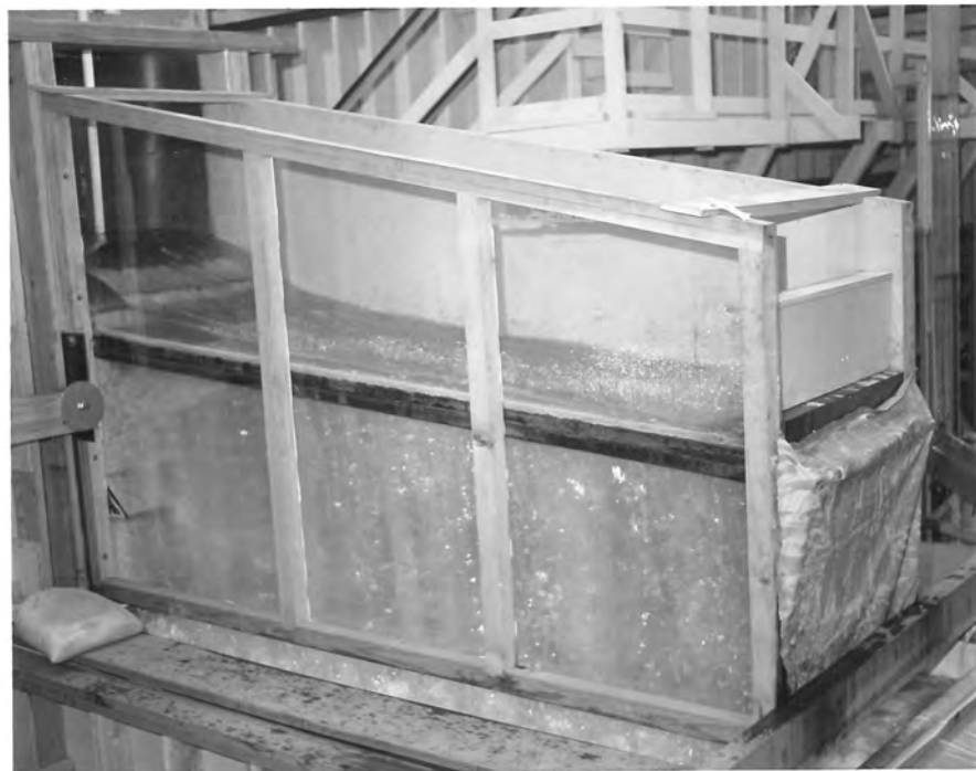
Figure 2. - Screen in sectional model. Flow is from left to right.
