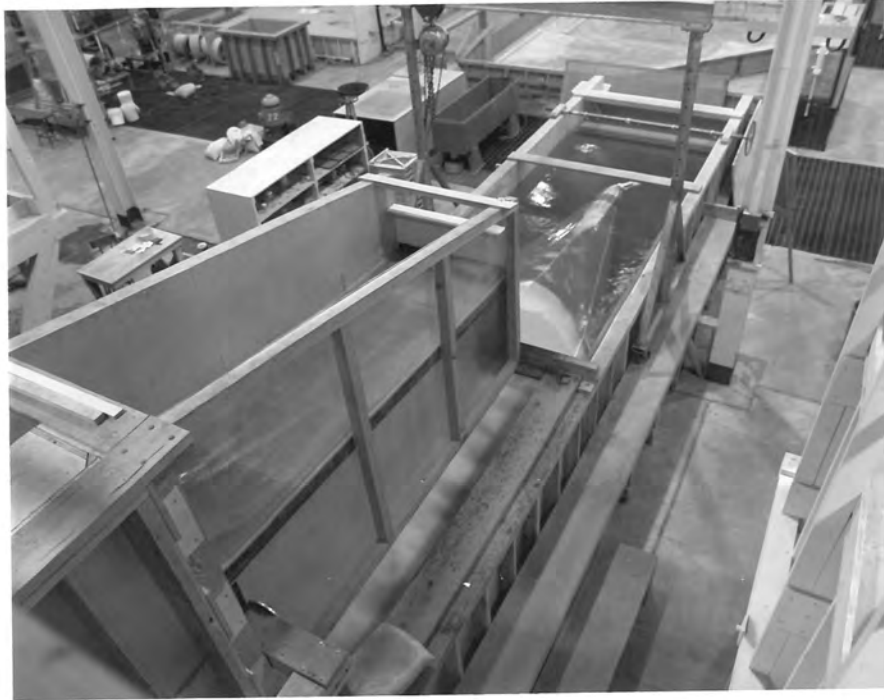
Figure 1. - Overall view of full-scale section model, looking downstream. Plankton net is visible in tailbox.
