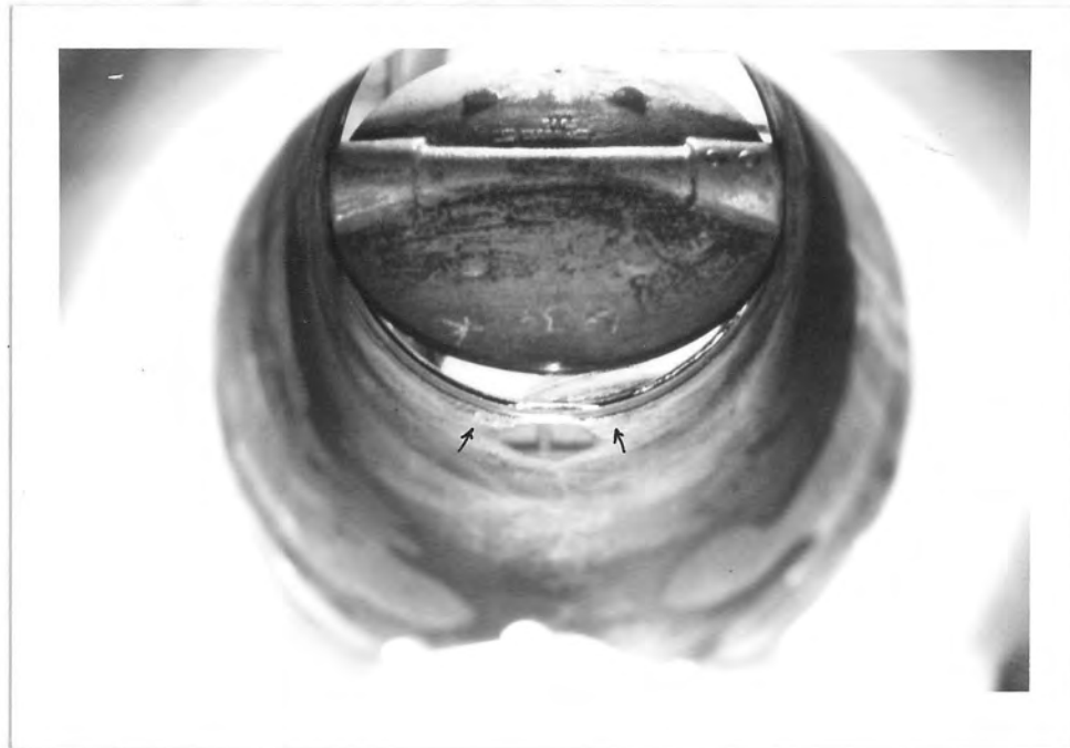
CAVITATION EROSION ON INVERT - FROM UPSTREAM SIDE OF CONTROLLER
