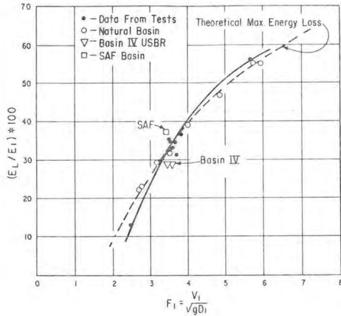
FIGURE 1-ENERGY LOSS COMPARED TO INCOMING ENERGY
