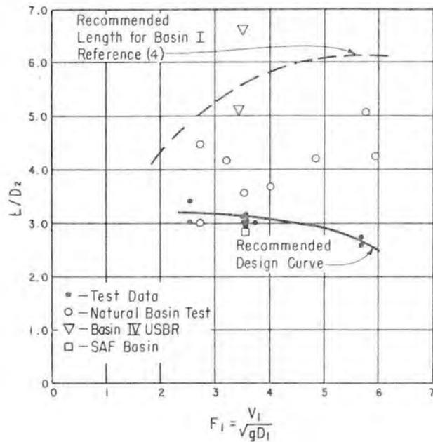
FIGURE 2-DIMENSIONLESS LENGTH OF STILLING BASIN
