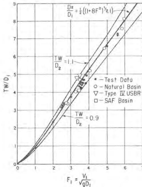
FIGURE 3-RATIO OF TAILWATER TO INFLOW DEPTH
