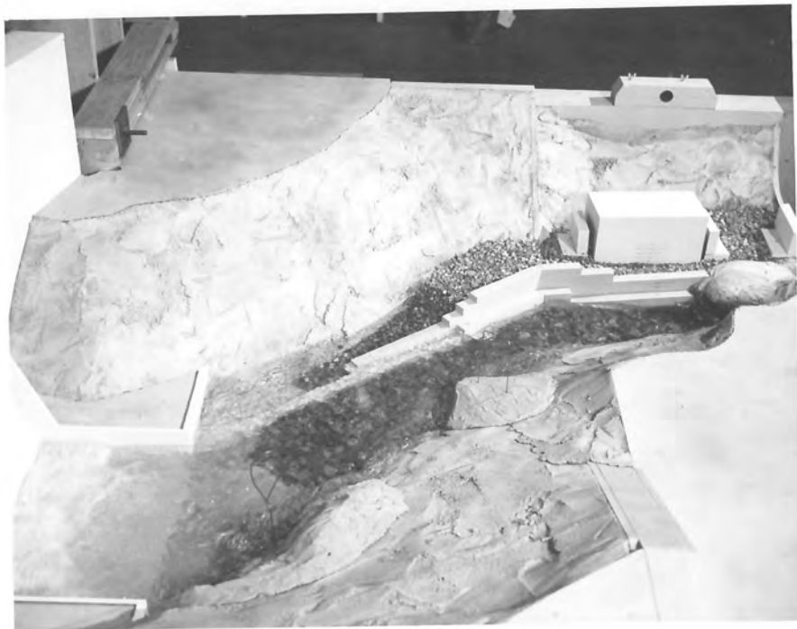
Figure 10. - Flow of 1,900 \text{ ft}^3/\text{s} , channel with topography features in place.
