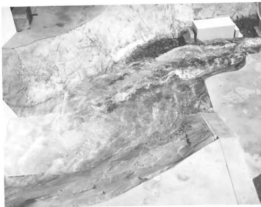
Figure 18. - Flow at 13,300 \text{ ft}^3/\text{s} with canyon wall, nob and rock removed.
