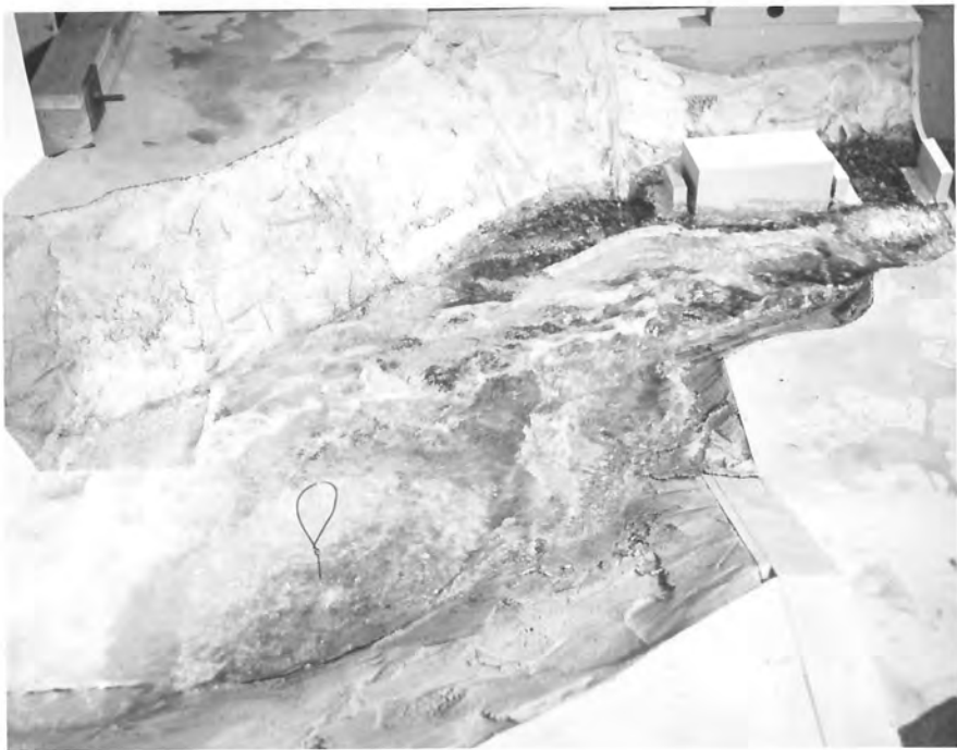
Figure 17. - Flow of 13,300 \text{ ft}^3/\text{s} with nob and rock removed.
