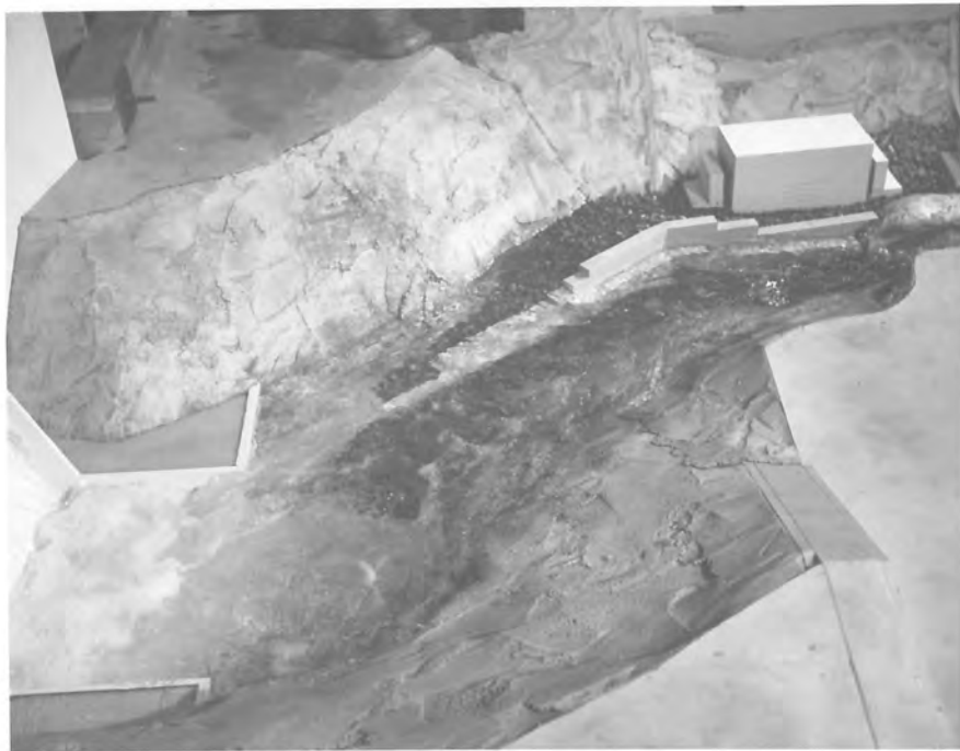
Figure 15. - Flow of 5,800 \text{ ft}^3/\text{s} , canyon wall, nob and rock removed.
