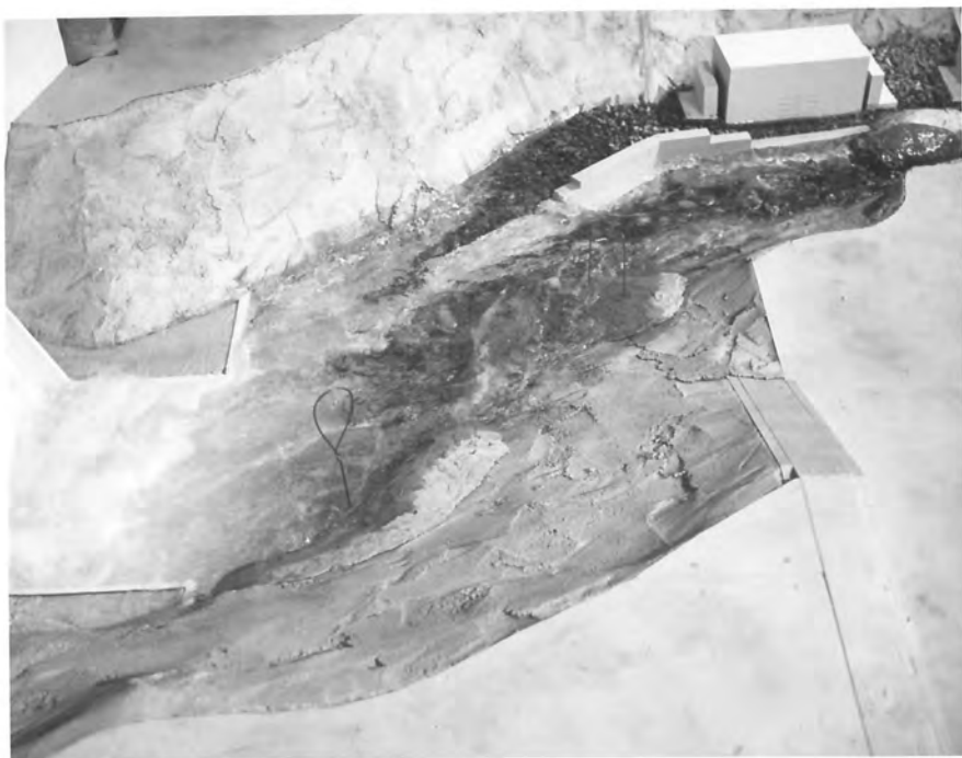
Figure 13. - Flow of 5,800 \text{ ft}^3/\text{s} , nob in place.
