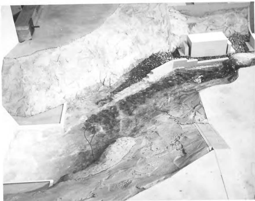
Figure 12. - Flow of 4,400 \text{ ft}^3/\text{s} , nob removed.
