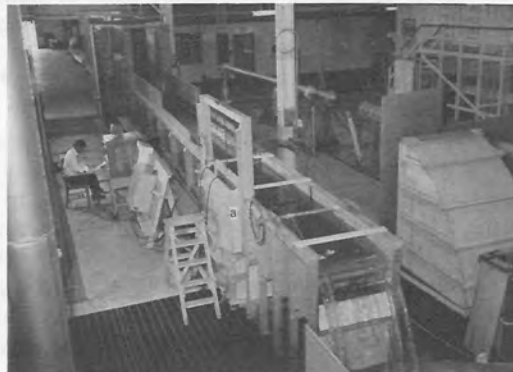
FIG. 3.—Laboratory Channel Installation of Ultrasonic Flowmeter: (a) Transducer Section of Channel
