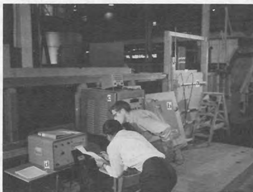
FIG. 5.—Ultrasonic Flowmeter Installation: (a) Transducer Section; (b) Flowmeter Electronics; (c) Integrating Digital Voltmeter; (d) Tape Printer
