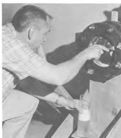
Figure 2G. Soap solution being applied to seal area to help locate air leakage if present. Photo P801-D-74491
