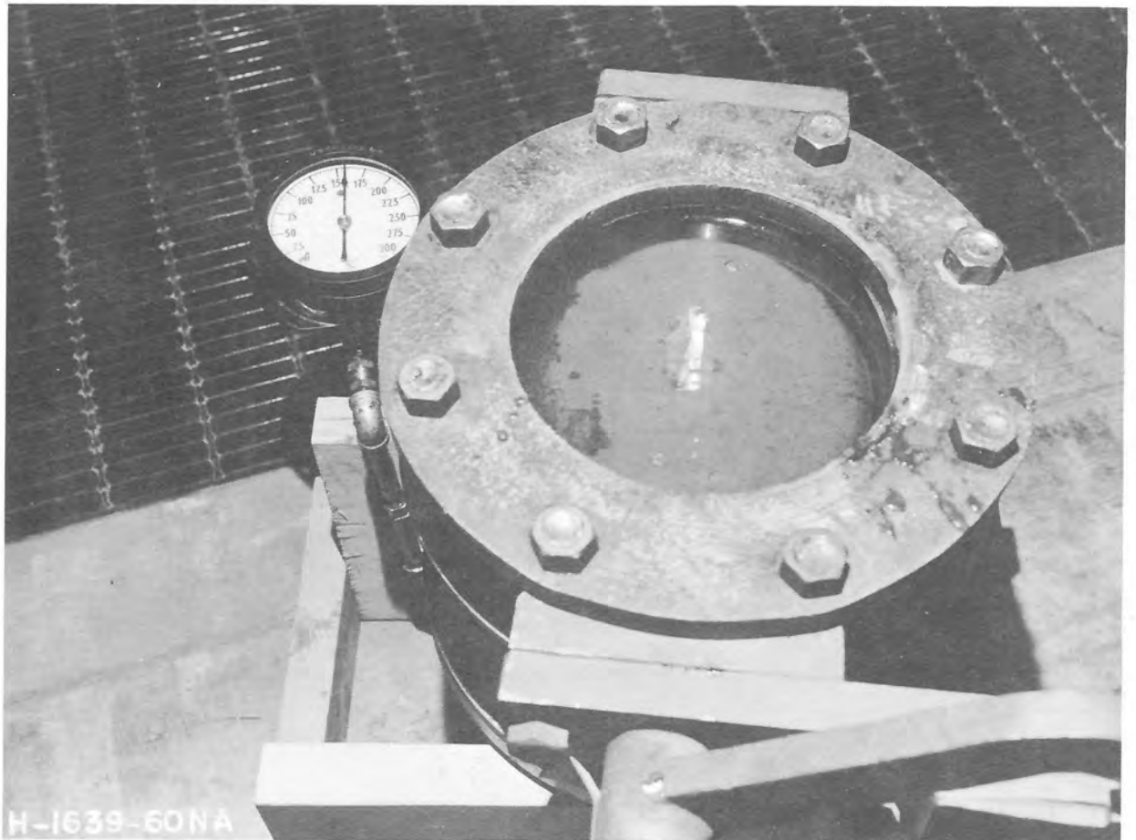
Figure 9AC. Bubble tightness tests on Allis-Chalmers valve after 4,000 cycles of opening and closing. Air at 156 psig (10.97 kg/cm 2 ) under the leaf. Photo P801-D-74512
