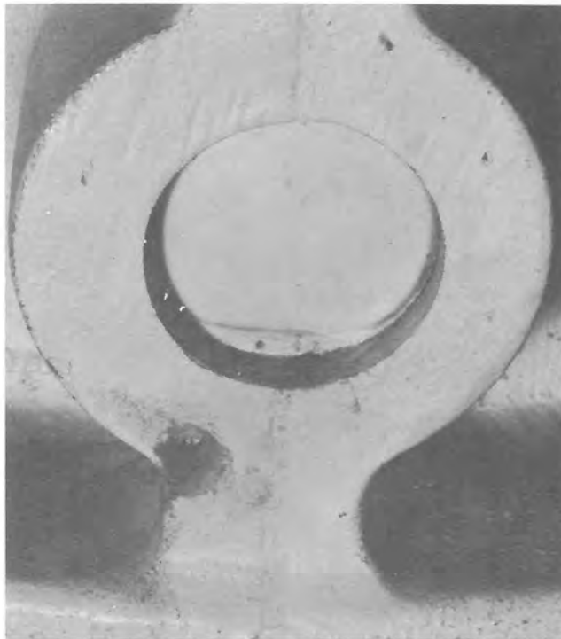
B. Location of shaft seal leakage. Photo P801-D-74500
