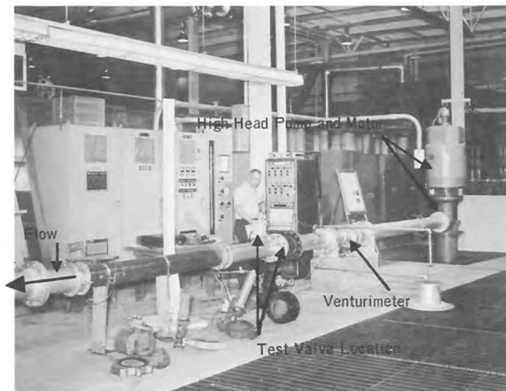
Figure 4G. Arrangement of high head test facility showing butterfly valve location. Photo P801-D-74493
