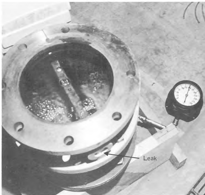
A. Leakage at 150 psig. Also note arrow showing leakage around shaft seal. Photo P801-D-74499
