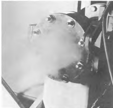
Figure 3G. Typical photo of a valve being opened with 70 to 90 psig air on the upstream side. Photo P801-D-74492
