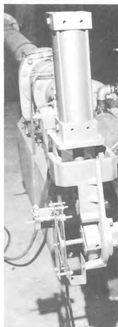
Figure 5GB. Potentiometer-gear system attached to Centerline valve. Photo P801-D-74495
