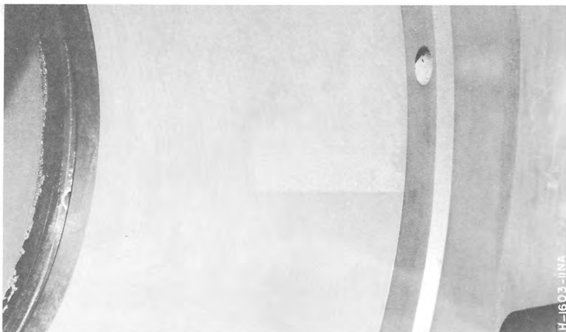
Figure 3. Closeup of right side of inlet cone and annular recess at throat. High-pressure pickup port at upper right, low-pressure port left center. Flow is from right to left. Photo PX-D-72452
