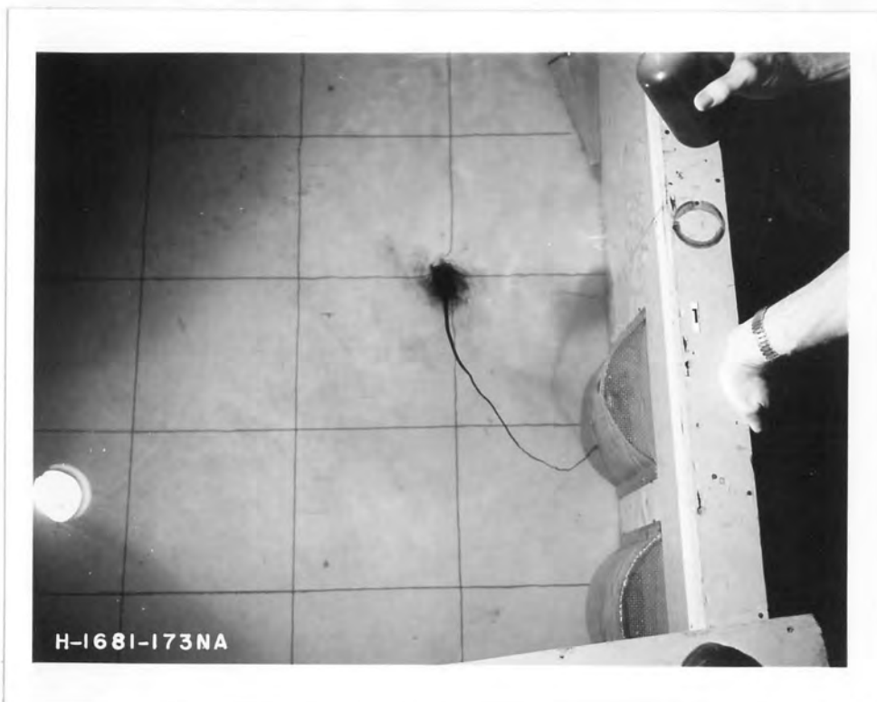
Figure 6. - Water surface elevation 1290 feet and units number 19, 23, and 24 operating, each with 3\frac{1}{3} times the model Froude Number discharge.
