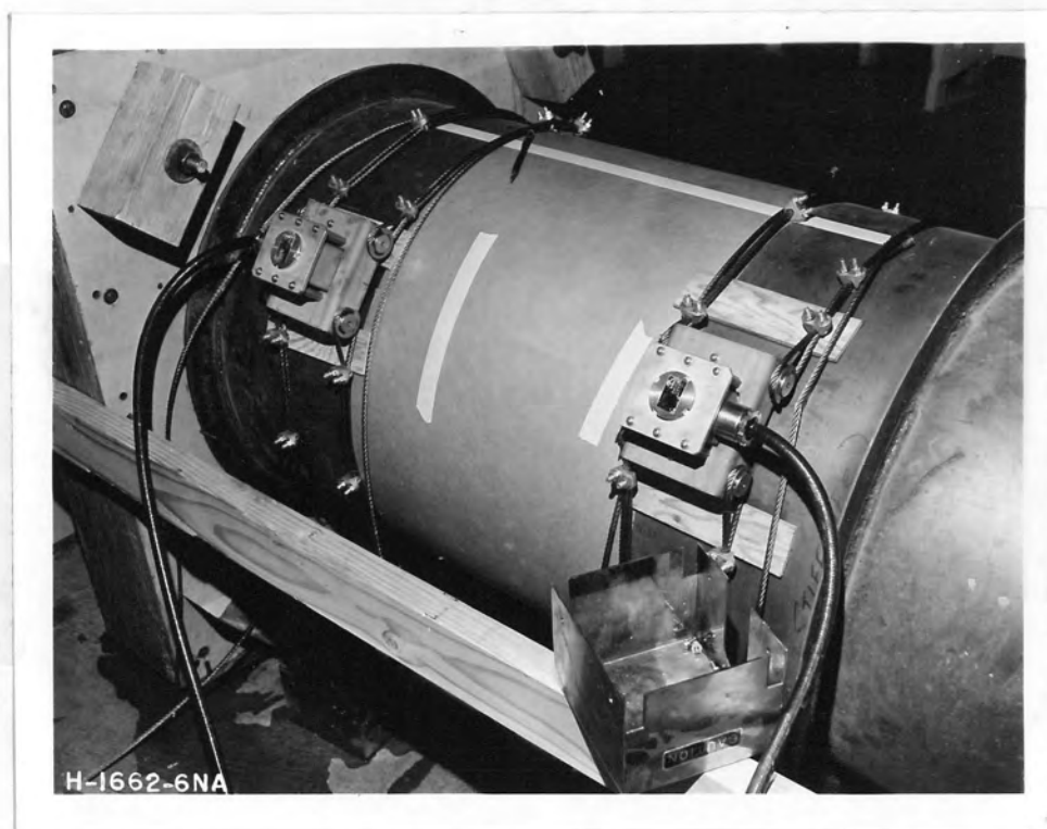
VIEW OF TRANSDUCERS INSTALLED ON STEEL PIPE (FLOW IS FROM LEFT TO RIGHT)
