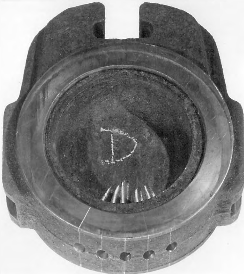
b. View of The Drilled Valve Disc
